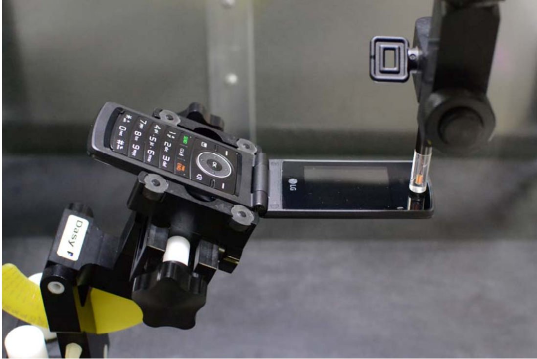
Figure 13-1 Test Setup for Wireless Device
