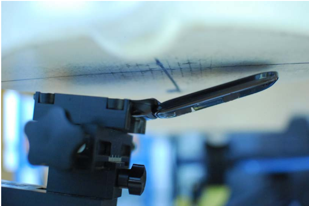
SAR Test Setup Photo 2 - Mouth Jaw Replacing Left Cheek
