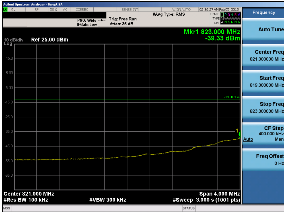
Plot 6-206. Lower Extended Band Edge Plot (Band 5 – 3.0MHz QPSK – RB Size 15)
