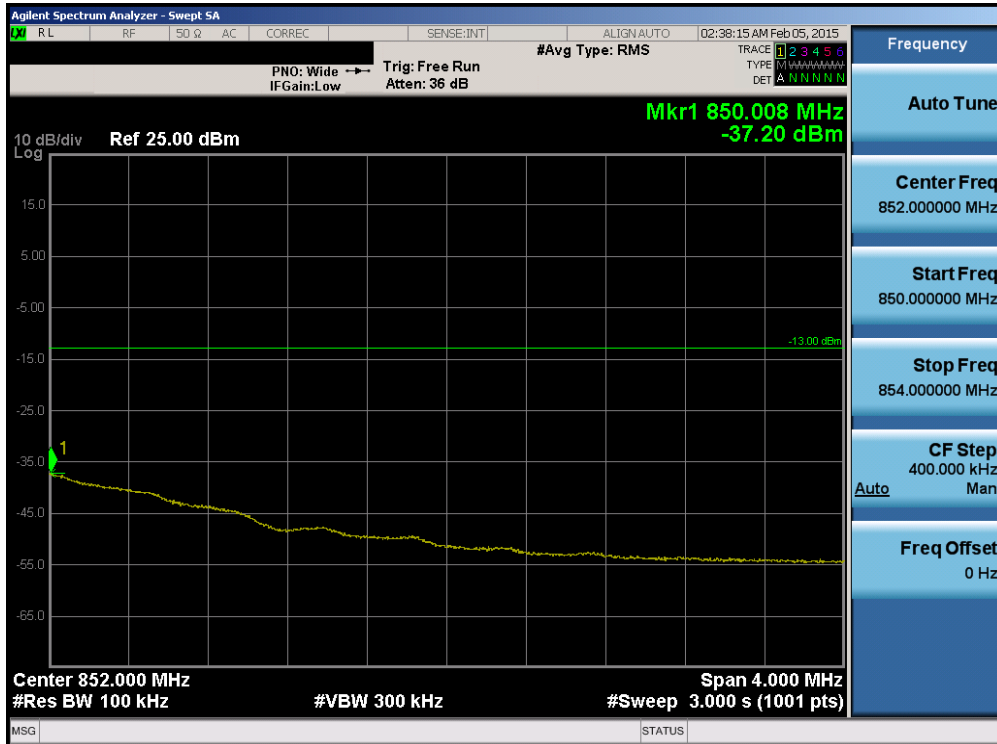
Plot 6-208. Upper Extended Band Edge Plot (Band 5 - Band 5 - 3.0MHz QPSK - RB Size 15)
