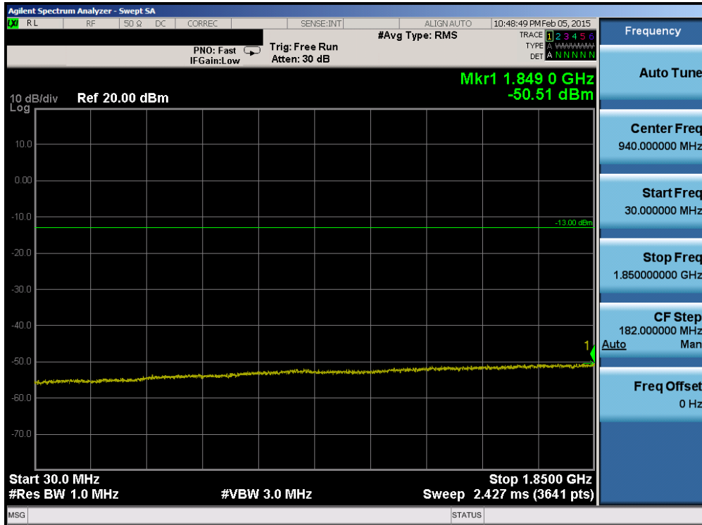
Plot 6-163. Conducted Spurious Plot (Band 2 – 5.0MHz QPSK – RB Size 1, RB Offset 0 – High Channel)
