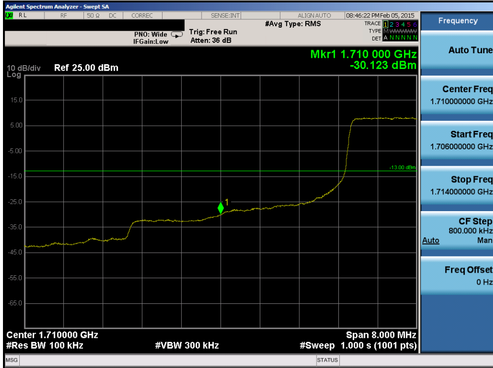
Plot 6-229. Lower Band Edge Plot (Band 4 – 10.0MHz QPSK – RB Size 50)
