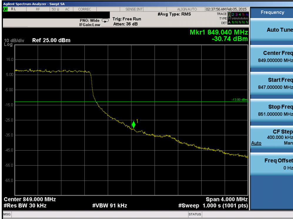
Plot 6-207. Upper Band Edge Plot (Band 5 - 3.0MHz QPSK - RB Size 15)
