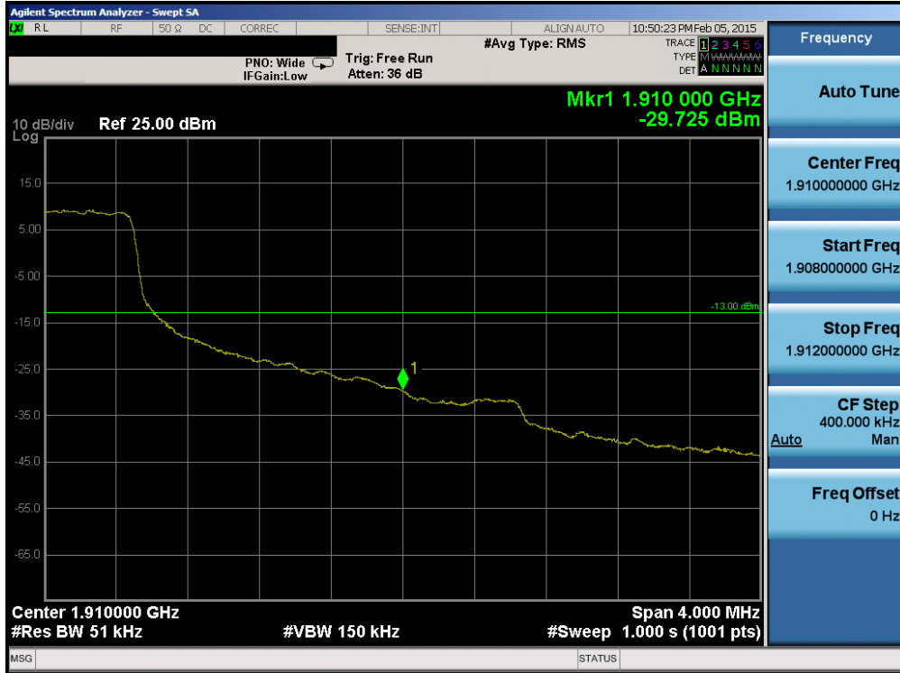
Plot 6-251. Upper Band Edge Plot (Band 2 – 5.0MHz QPSK – RB Size 25)
