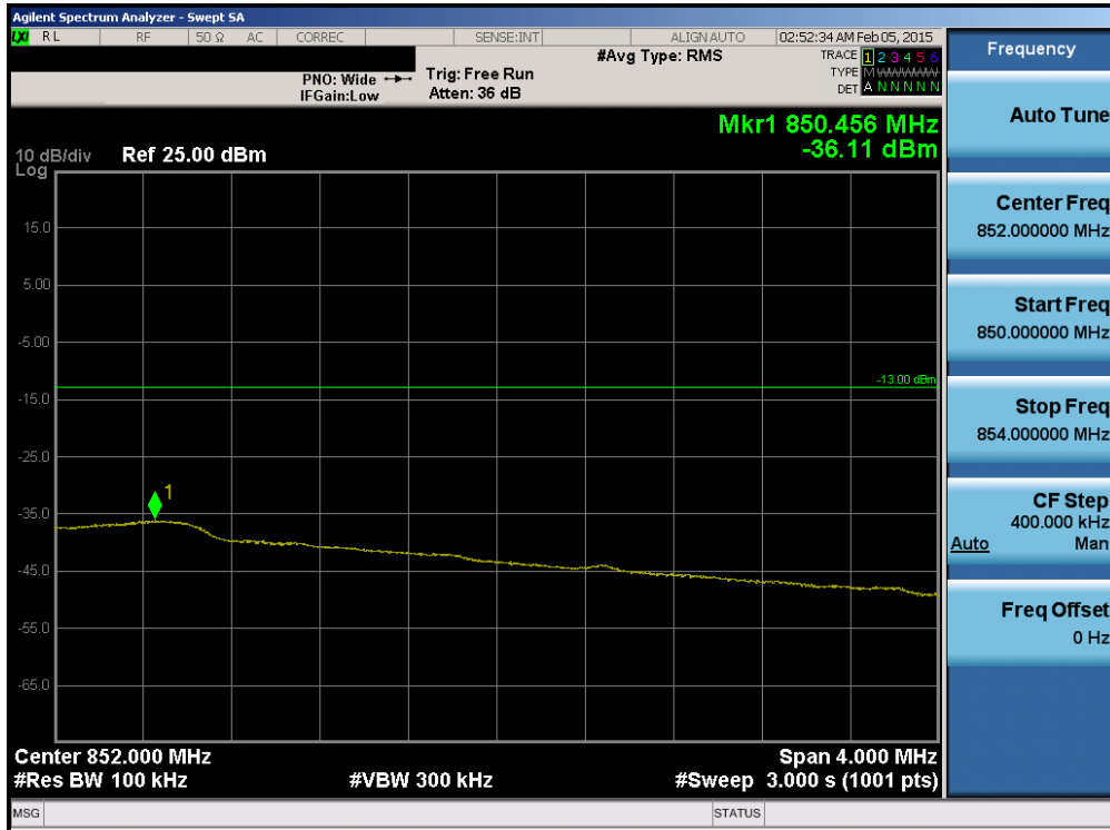
Plot 6-216. Upper Extended Band Edge Plot (Band 5 – 10.0MHz QPSK – RB Size 50)
