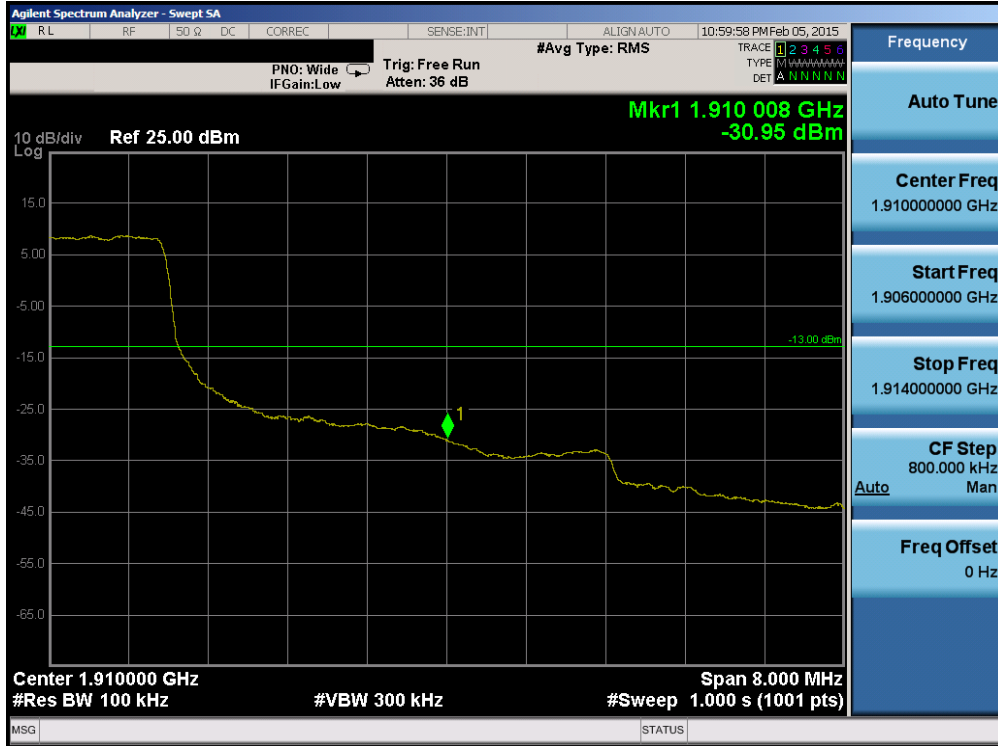
Plot 6-255. Upper Band Edge Plot (Band 2 – 10.0MHz QPSK – RB Size 50)
