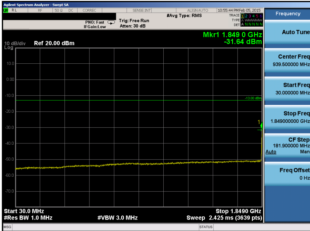
Plot 6-166. Conducted Spurious Plot (Band 2 – 10.0MHz QPSK – RB Size 1, RB Offset 0– Low Channel)
