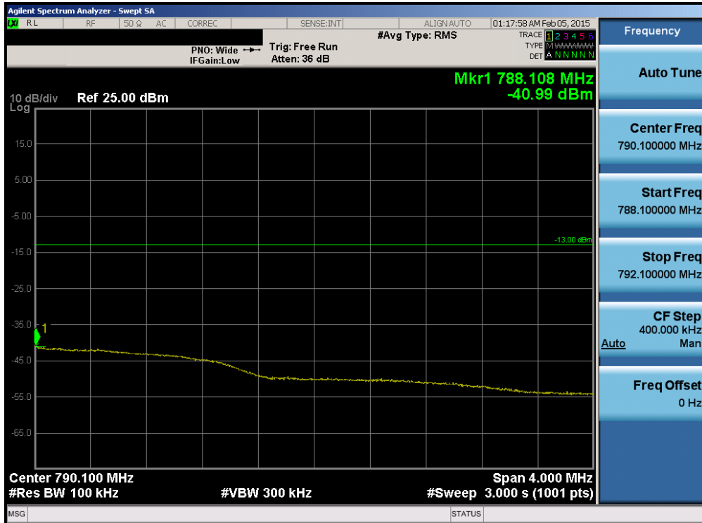
Plot 6-196. Upper Extended Band Edge Plot (Band 13 – 5.0MHz QPSK – RB Size 25)
