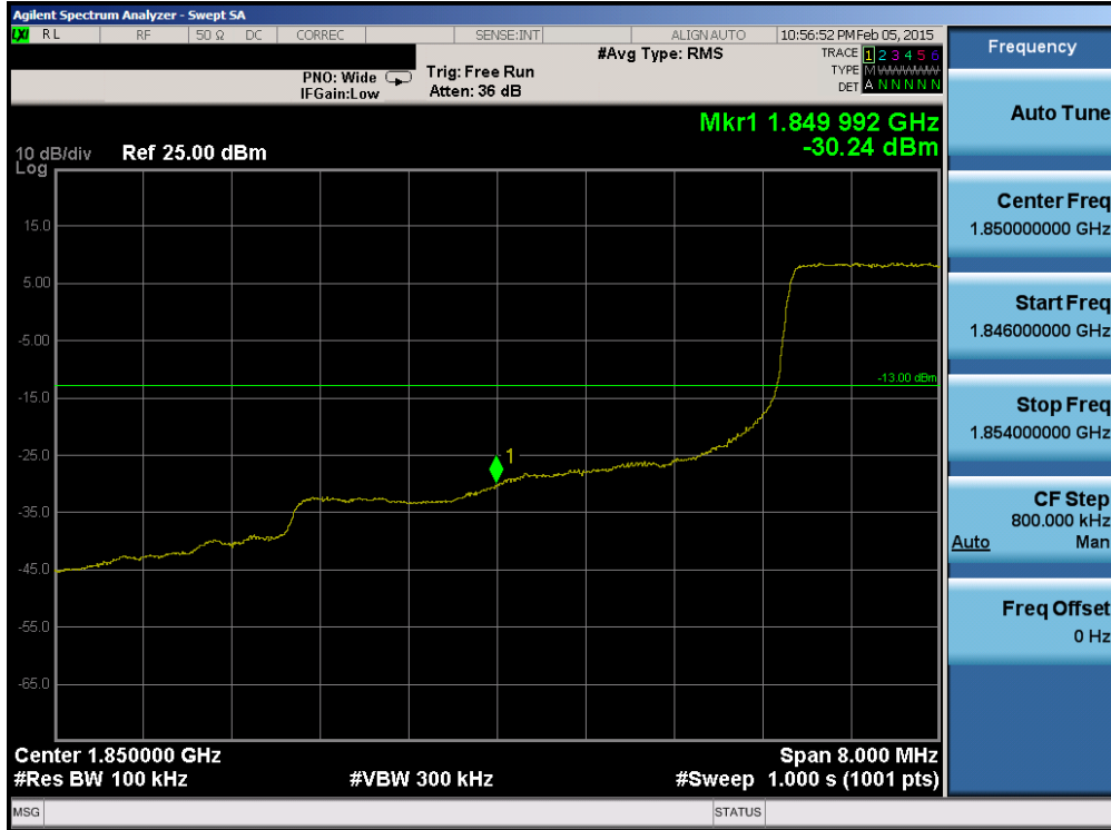
Plot 6-253. Lower Band Edge Plot (Band 2 – 10.0MHz QPSK – RB Size 50)
