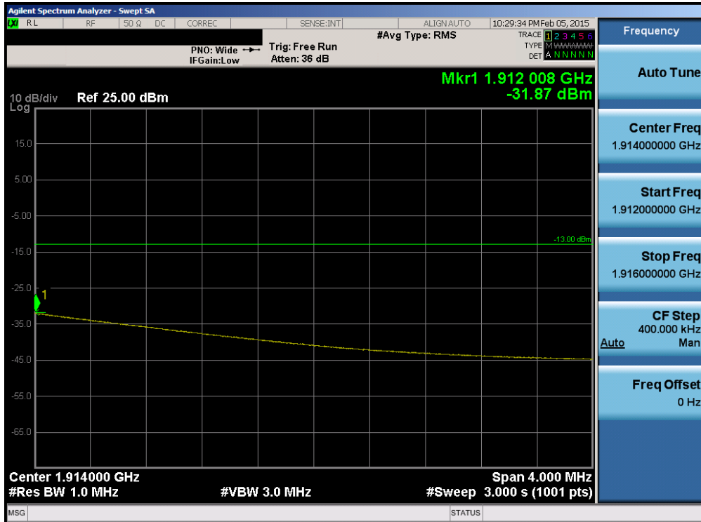
Plot 6-244. Upper Extended Band Edge Plot (Band 2 – 1.4MHz QPSK – RB Size 6)
