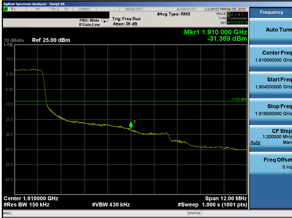
Plot 6-259. Upper Band Edge Plot (Band 2 – 15.0MHz QPSK – RB Size 75)
