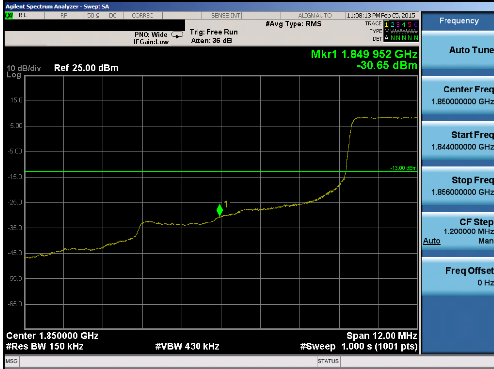
Plot 6-257. Lower Band Edge Plot (Band 2 – 15.0MHz QPSK – RB Size 75)
