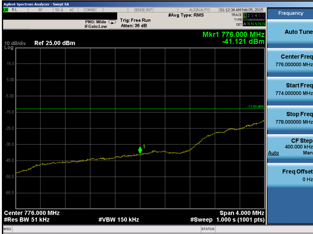
Plot 6-193. Lower Band Edge Plot (Band 13 – 5.0MHz QPSK – RB Size 25)
