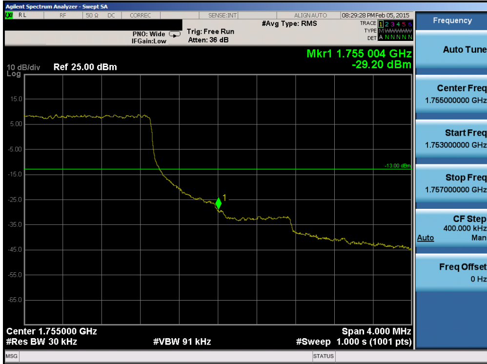
Plot 6-223. Upper Band Edge Plot (Band 4 – 3.0MHz QPSK – RB Size 15)
