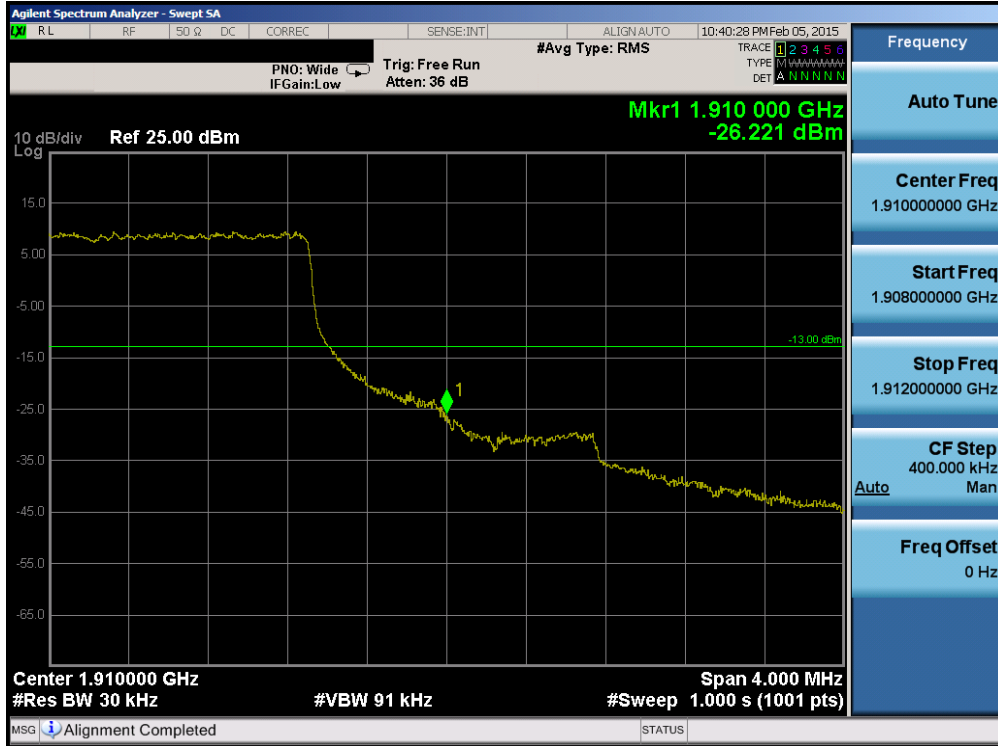
Plot 6-247. Upper Band Edge Plot (Band 2 – 3.0MHz QPSK – RB Size 15)
