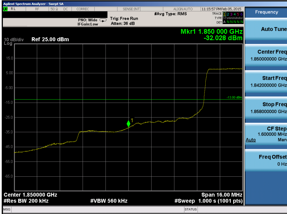
Plot 6-261. Lower Band Edge Plot (Band 2 – 20.0MHz QPSK – RB Size 100)
