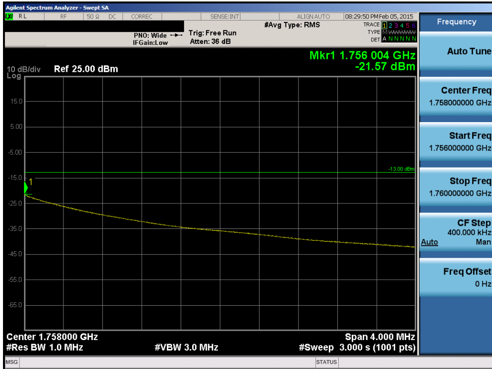
Plot 6-220. Upper Extended Band Edge Plot (Band 4 – 1.4MHz QPSK – RB Size 6)
