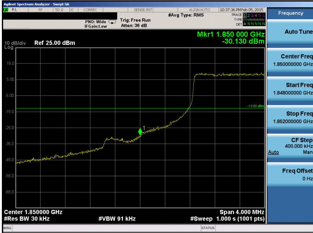
Plot 6-245. Lower Band Edge Plot (Band 2 – 3.0MHz QPSK – RB Size 15)
