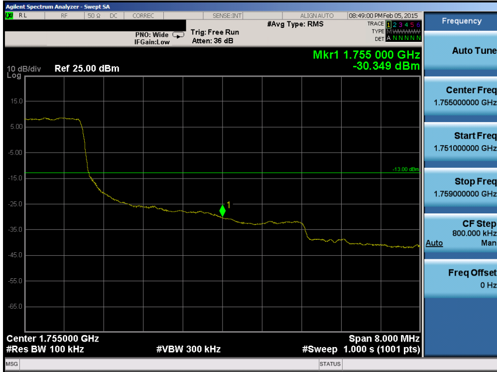
Plot 6-231. Upper Band Edge Plot (Band 4 – 10.0MHz QPSK – RB Size 50)
