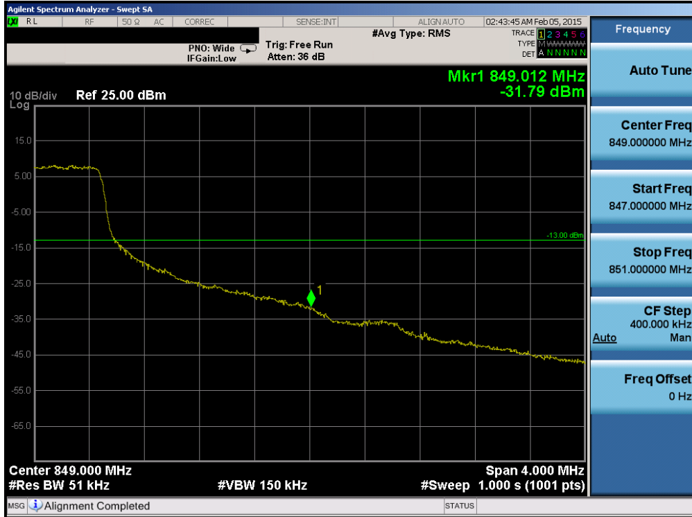
Plot 6-211. Upper Band Edge Plot (Band 5 - 5.0MHz QPSK - RB Size 25)
