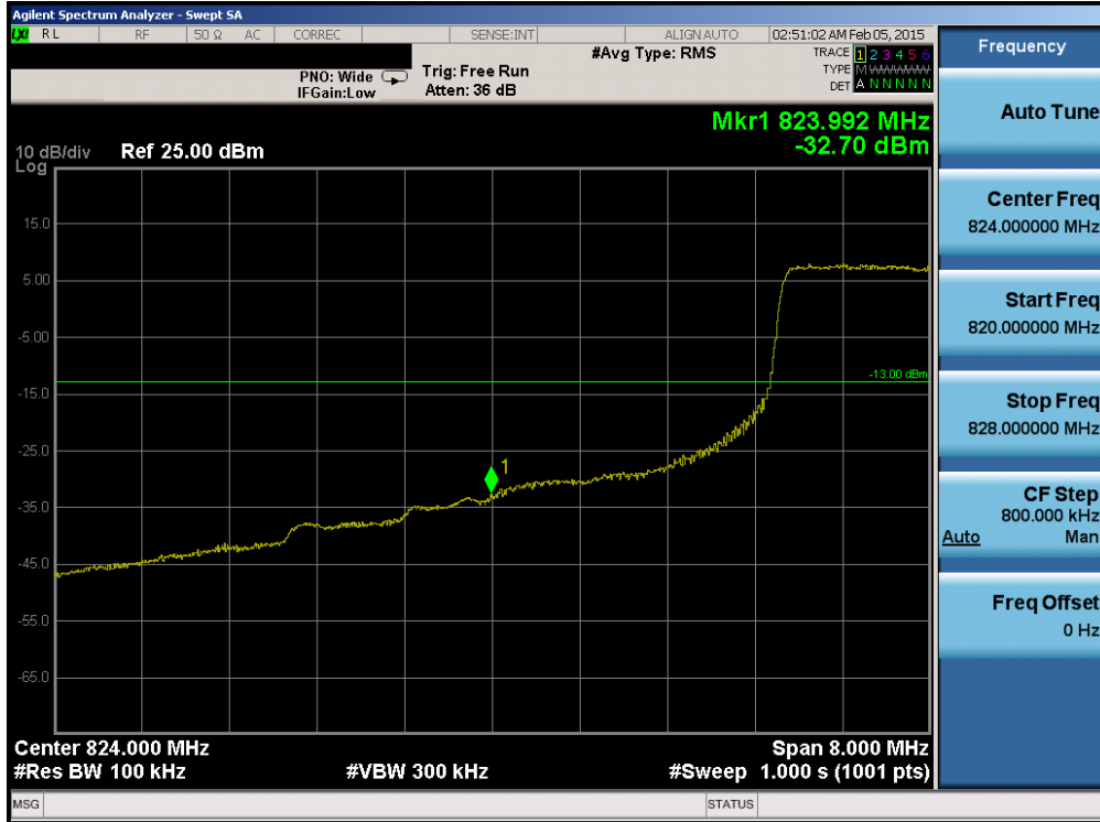
Plot 6-213. Lower Band Edge Plot (Band 5 – 10.0MHz QPSK – RB Size 50)
