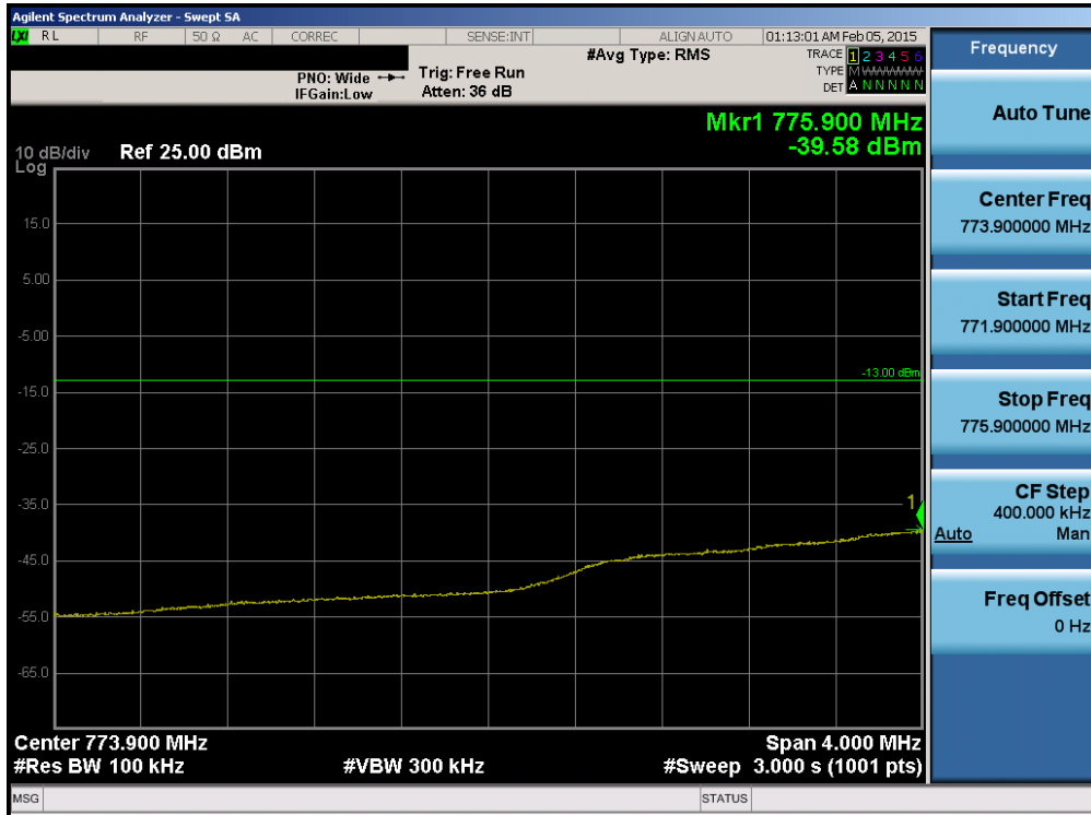
Plot 6-194. Lower Extended Band Edge Plot (Band 13 – 5.0MHz QPSK – RB Size 25)
