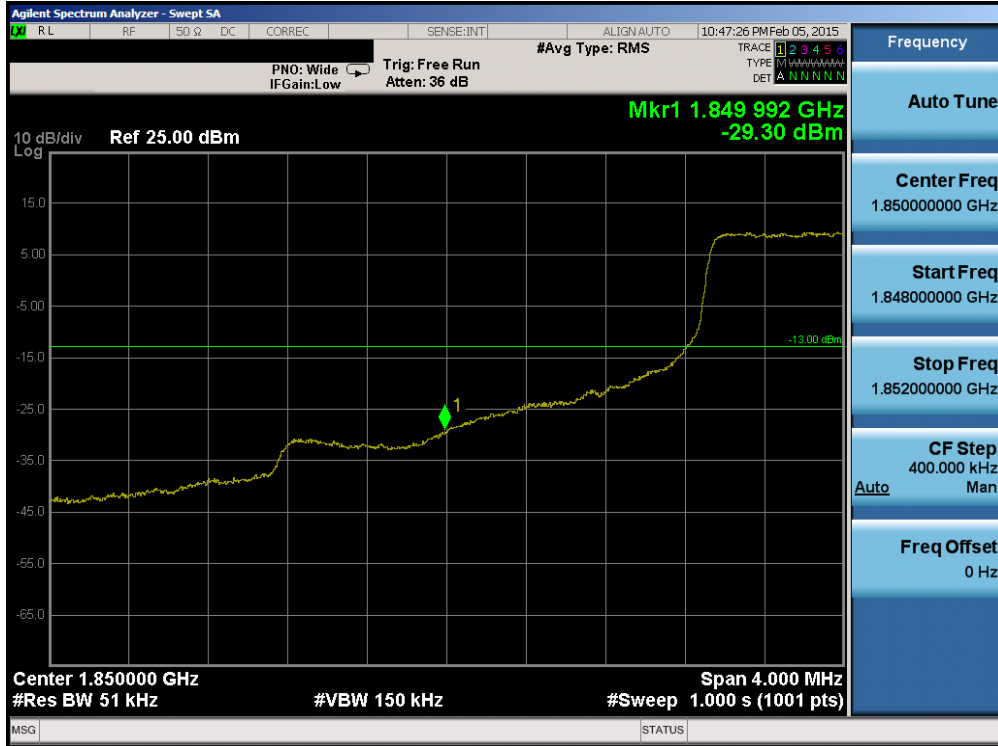
Plot 6-249. Lower Band Edge Plot (Band 2 – 5.0MHz QPSK – RB Size 25)
