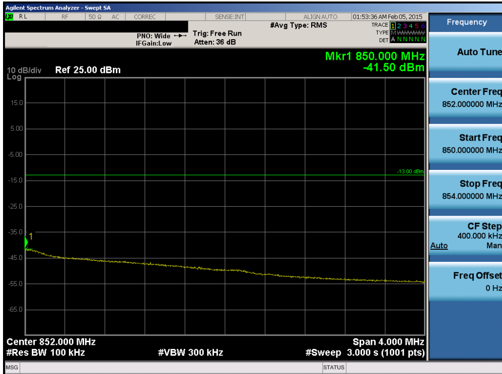
Plot 6-204. Upper Extended Band Edge Plot (Band 5 – 1.4MHz QPSK – RB Size 6)
