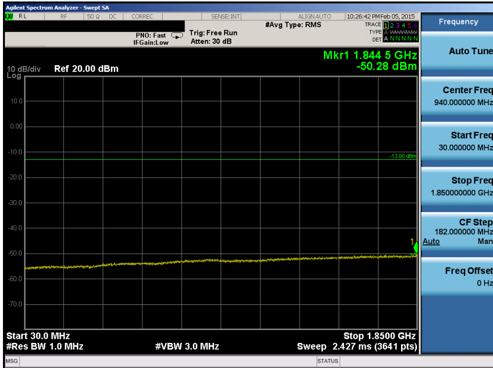
Plot 6-145. Conducted Spurious Plot (Band 2 – 1.4MHz QPSK – RB Size 1, RB Offset 0 – High Channel)
