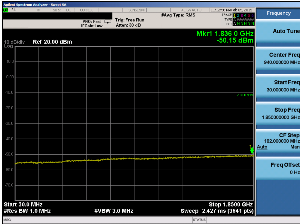
Plot 6-187. Conducted Spurious Plot (Band 2 – 20.0MHz QPSK – RB Size 1, RB Offset 0 – Mid Channel)
