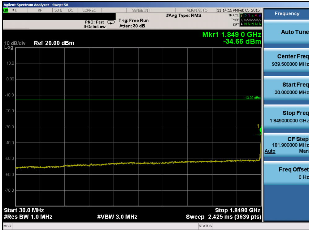
Plot 6-184. Conducted Spurious Plot (Band 2 – 20.0MHz QPSK – RB Size 1, RB Offset 0– Low Channel)
