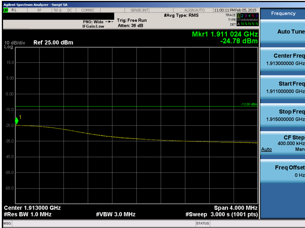
Plot 6-256. Upper Extended Band Edge Plot (Band 2 – 10.0MHz QPSK – RB Size 50)
