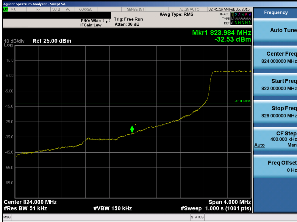
Plot 6-209. Lower Band Edge Plot (Band 5 – 5.0MHz QPSK – RB Size 25)
