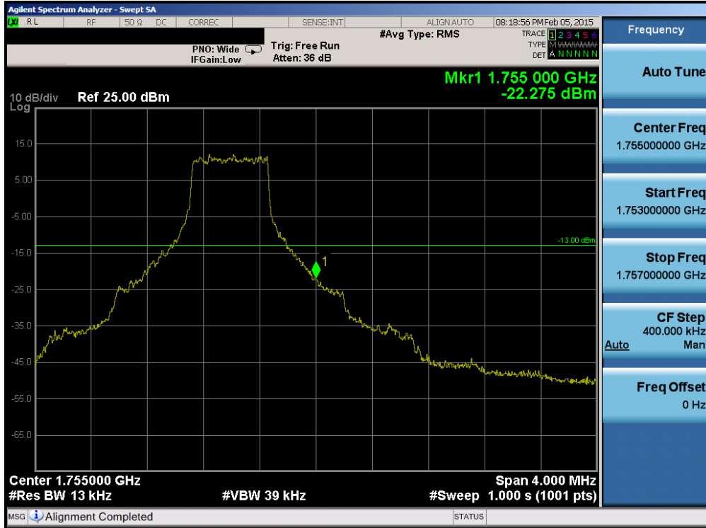
Plot 6-219. Upper Band Edge Plot (Band 4 – 1.4MHz QPSK – RB Size 6)
