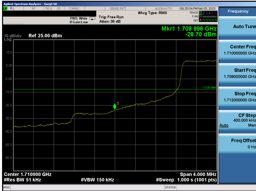
Plot 6-225. Lower Band Edge Plot (Band 4 – 5.0MHz QPSK – RB Size 25)
