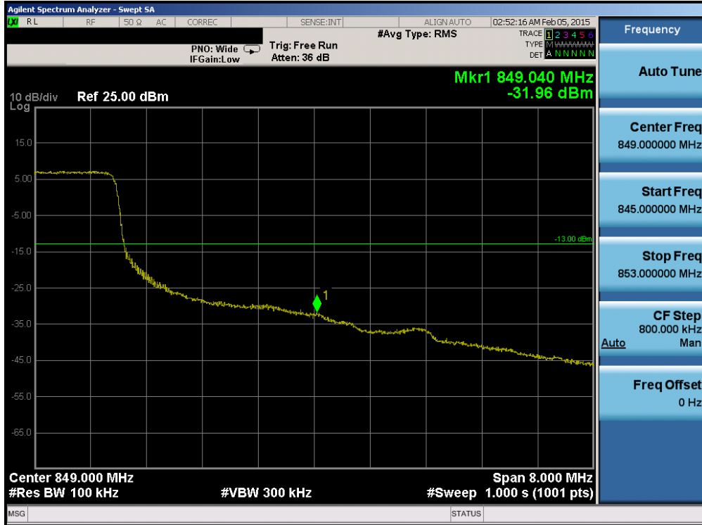
Plot 6-215. Upper Band Edge Plot (Band 5 – 10.0MHz QPSK – RB Size 50)
