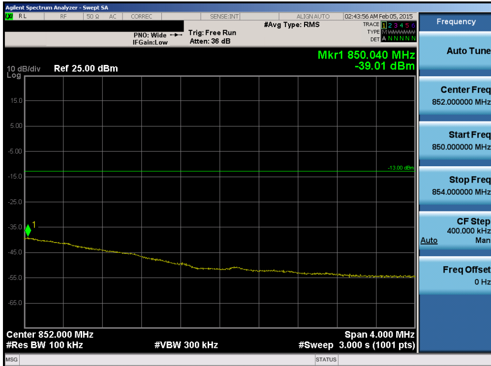
Plot 6-212. Upper Extended Band Edge Plot (Band 5 - 5.0MHz QPSK - RB Size 25)
