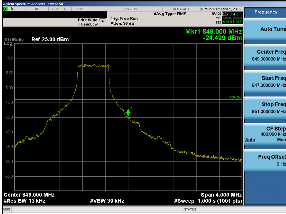
Plot 6-203. Upper Band Edge Plot (Band 5 – 1.4MHz QPSK – RB Size 6)
