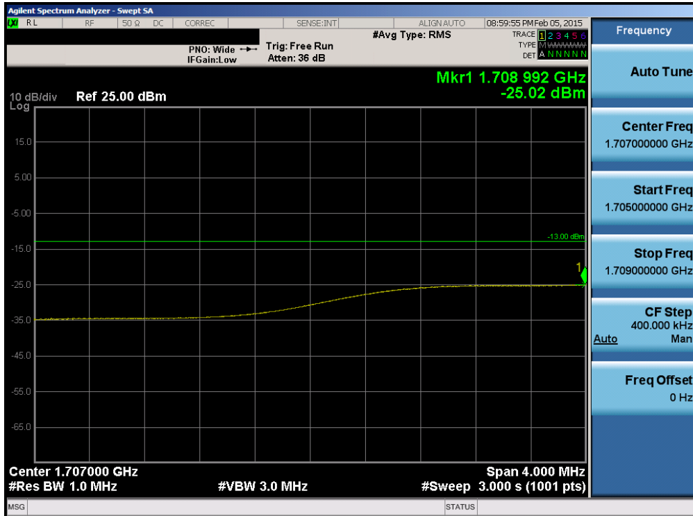
Plot 6-234. Lower Extended Band Edge Plot (Band 4 – 15.0MHz QPSK – RB Size 75)
