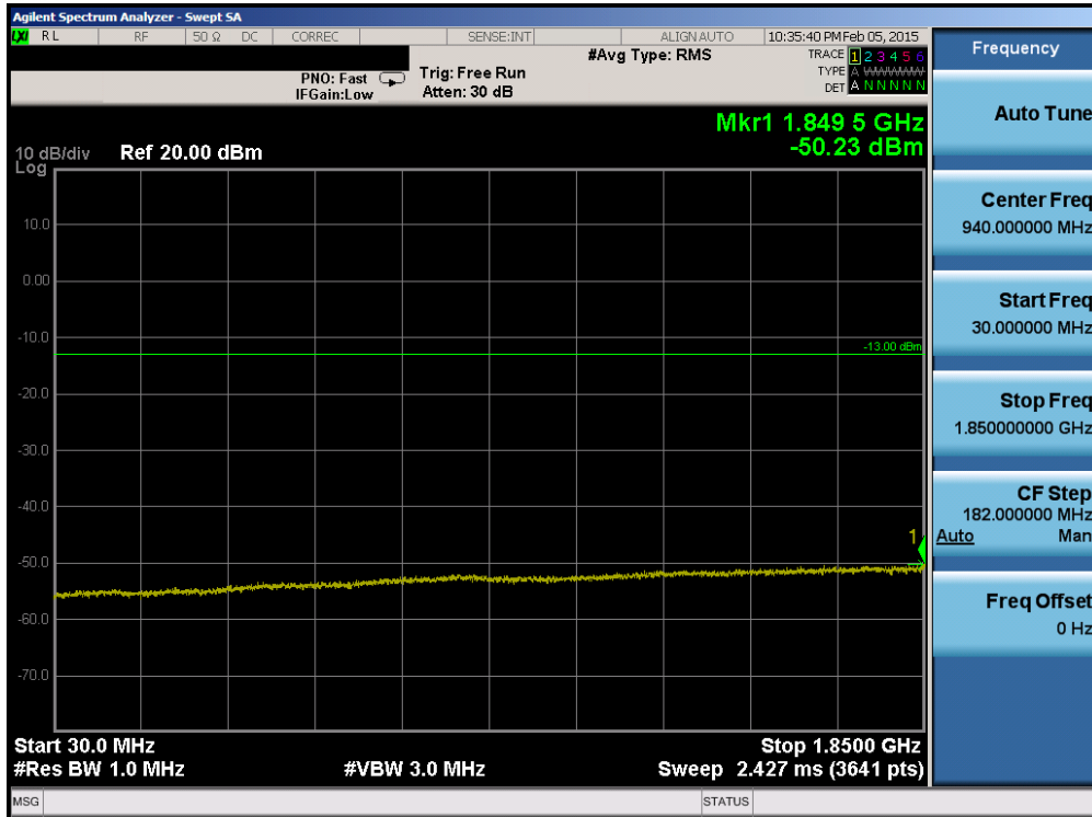
Plot 6-151. Conducted Spurious Plot (Band 2 – 3.0MHz QPSK – RB Size 1, RB Offset 0 – Mid Channel)
