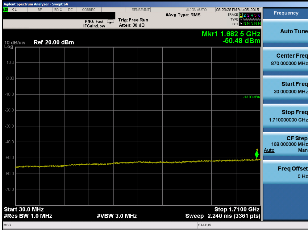
Plot 6-97. Conducted Spurious Plot (Band 4 – 3.0MHz QPSK – RB Size 1, RB Offset 0 – Mid Channel)
