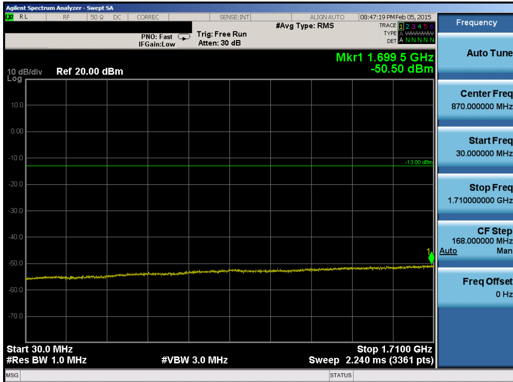
Plot 6-118. Conducted Spurious Plot (Band 4 – 10.0MHz QPSK – RB Size 1, RB Offset 0 – High Channel)
