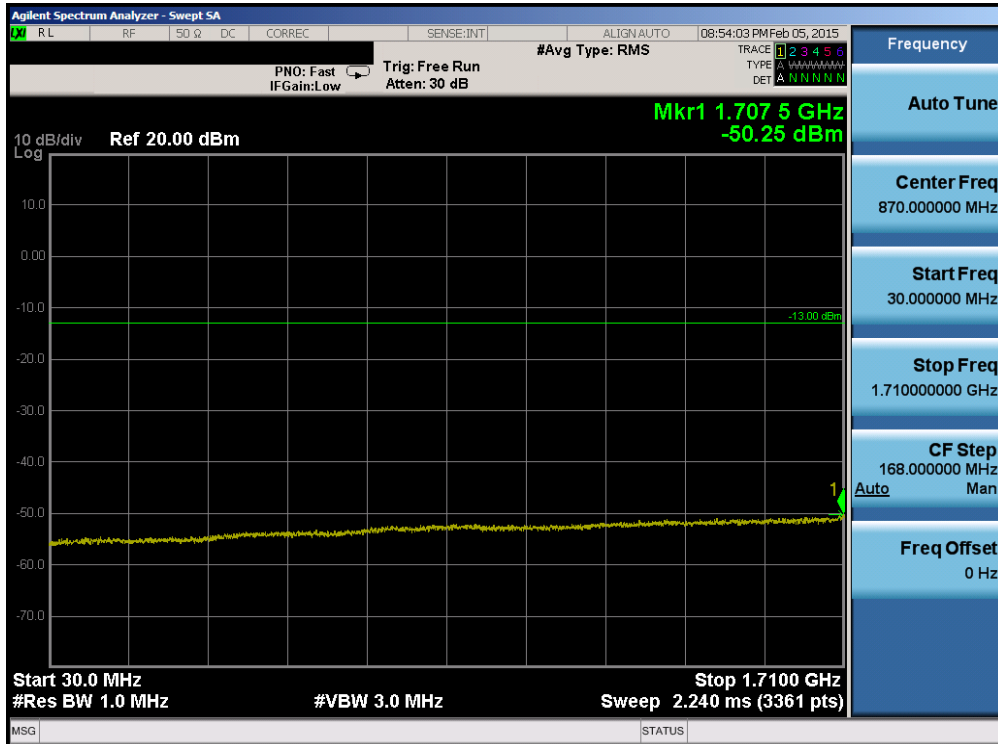
Plot 6-124. Conducted Spurious Plot (Band 4 – 15.0MHz QPSK – RB Size 1, RB Offset 0 – Mid Channel)
