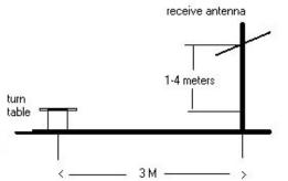
Figure 6-5. Test Instrument & Measurement Setup
