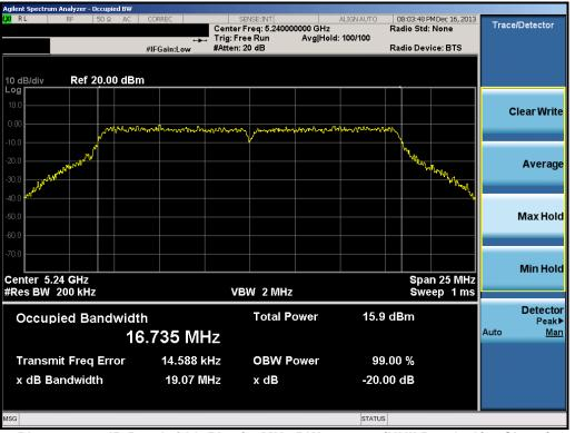
Plot 6-26. 20dB Bandwidth Plot (20MHz BW 802.11a (UNII Band 2A) - Ch. 48)
