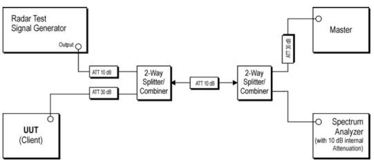
Figure 3-1. Conducted Test Setup for DFS
