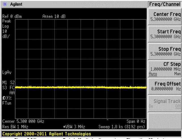
Figure 5-5 Non-occupancy Period - Monitoring live spectrum - Elapse time 30 minutes
