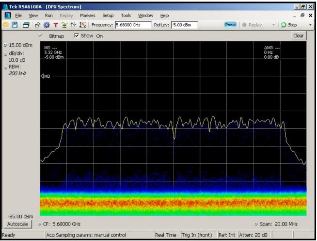
Figure 6-3. Real-Time Spectrum Display, WLAN Traffic (Streaming Video)
