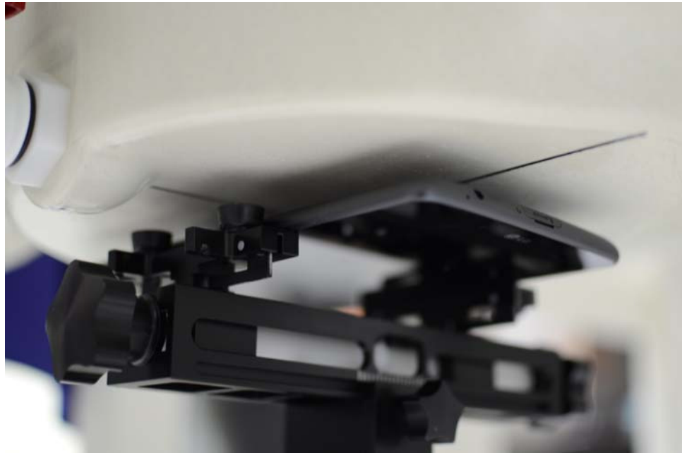
SAR Test Setup Photo 2: Back Side at 14 mm
