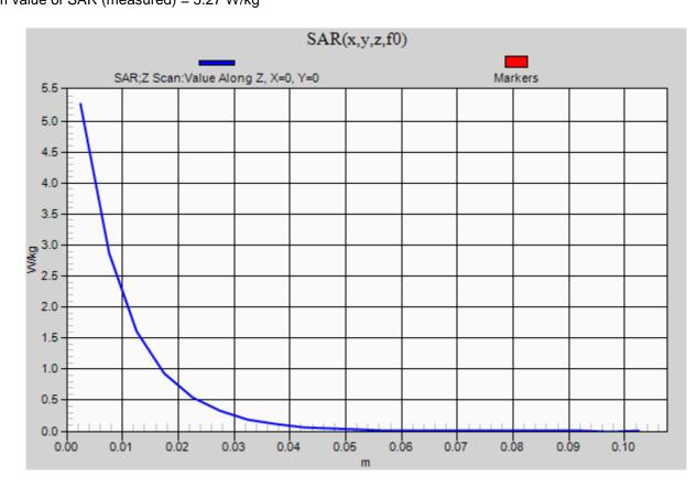
Frequency: 835 MHz; Duty Cycle: 1:1; Room Ambient Temperature: 24.0°C; Liquid Temperature: 23.0°C Medium parameters used: f = 835 MHz;  $\sigma$  = 1.017 S/m;  $\epsilon_r$  = 52.796;  $\rho$  = 1000 kg/m<sup>3</sup> DASY5 Configuration:
