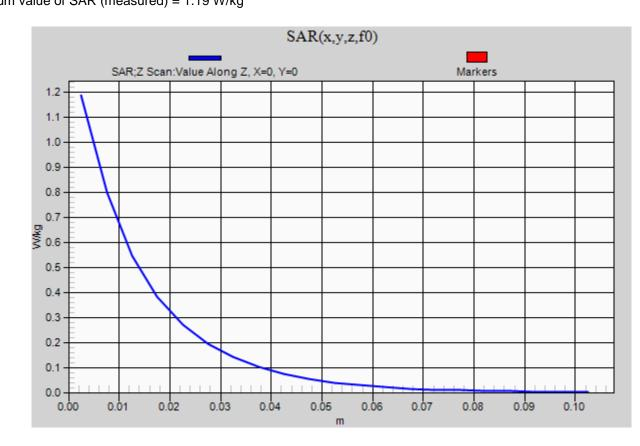
Frequency: 1900 MHz; Duty Cycle: 1:1; Room Ambient Temperature: 24.0°C; Liquid Temperature: 23.0°C Medium parameters used: f = 1900 MHz;  $\sigma$  = 1.416 S/m;  $\epsilon_r$  = 39.363;  $\rho$  = 1000 kg/m<sup>3</sup> DASY5 Configuration:
