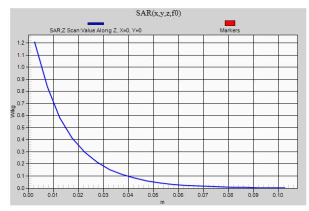
Frequency: 1900 MHz; Duty Cycle: 1:1; Room Ambient Temperature: 24.0°C; Liquid Temperature: 23.0°C Medium parameters used: f = 1900 MHz;  $\sigma$  = 1.529 S/m;  $\epsilon_r$  = 51.827;  $\rho$  = 1000 kg/m<sup>3</sup> DASY5 Configuration:
