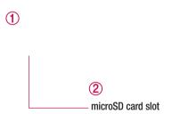
2 If you want to use a memory card, insert the memory card into the lower slot. Make sure the gold contact area is facing upwards. Slide the microSD card into the slot until it "clicks" into place and then close the slot cover.
