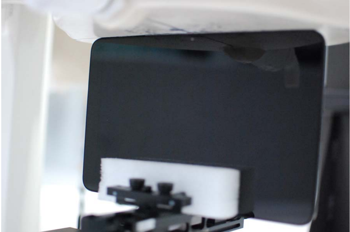
SAR Test Setup Photo 7: Right Edge at 0.0 cm
