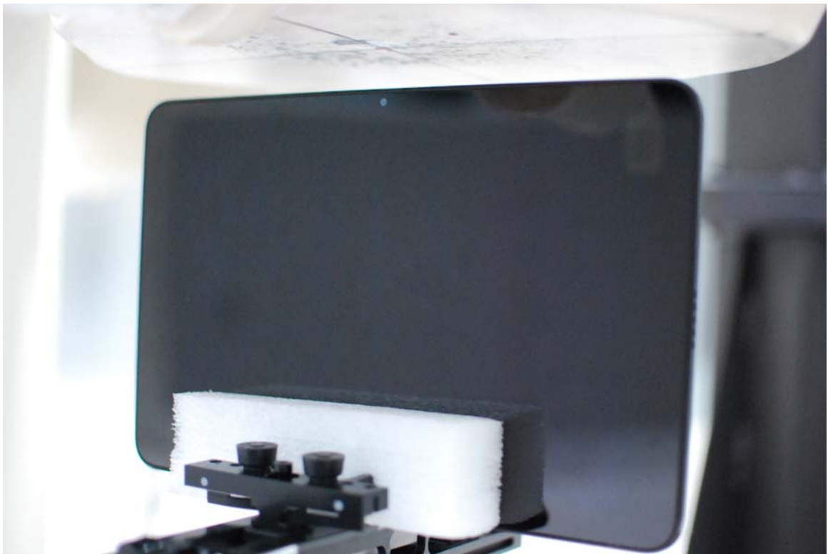
SAR Test Setup Photo 6: Right Edge at 1.4 cm
