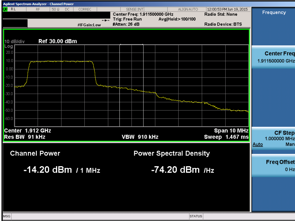
Plot 6-149. Upper Extended Band Edge Plot (Band 2 – 3.0MHz QPSK – RB Size 15)
