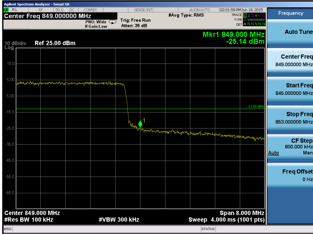
Plot 6-117. Upper Band Edge Plot (Band 5 – 10.0MHz QPSK – RB Size 50)
