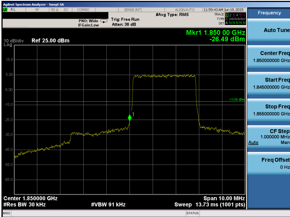
Plot 6-146. Lower Band Edge Plot (Band 2 – 3.0MHz QPSK – RB Size 15)
