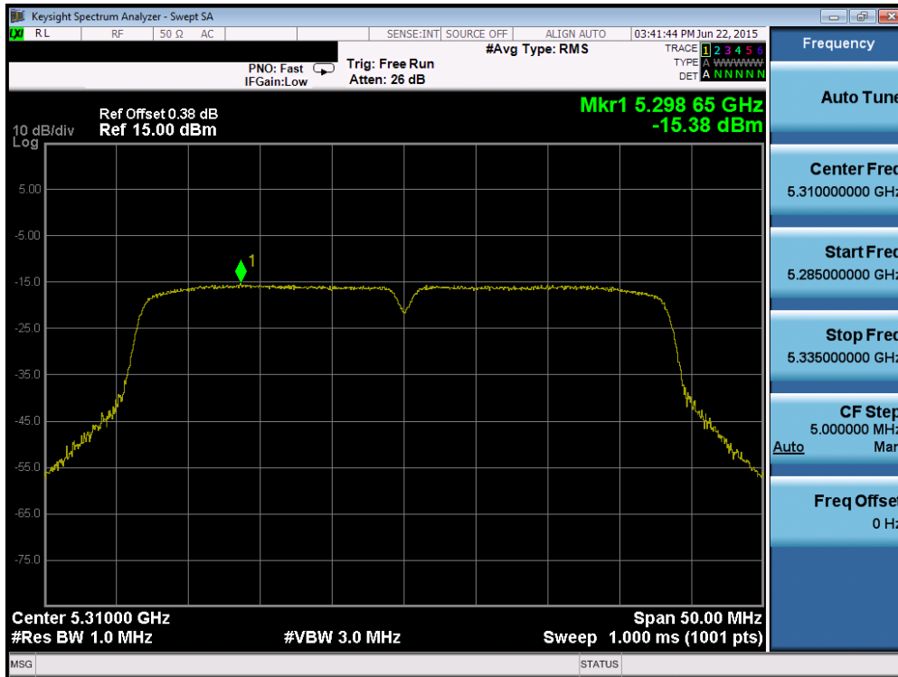
Plot 6-54. Power Spectral Density Plot (40MHz BW 802.11n (UNII Band 2A) – Ch. 62)
