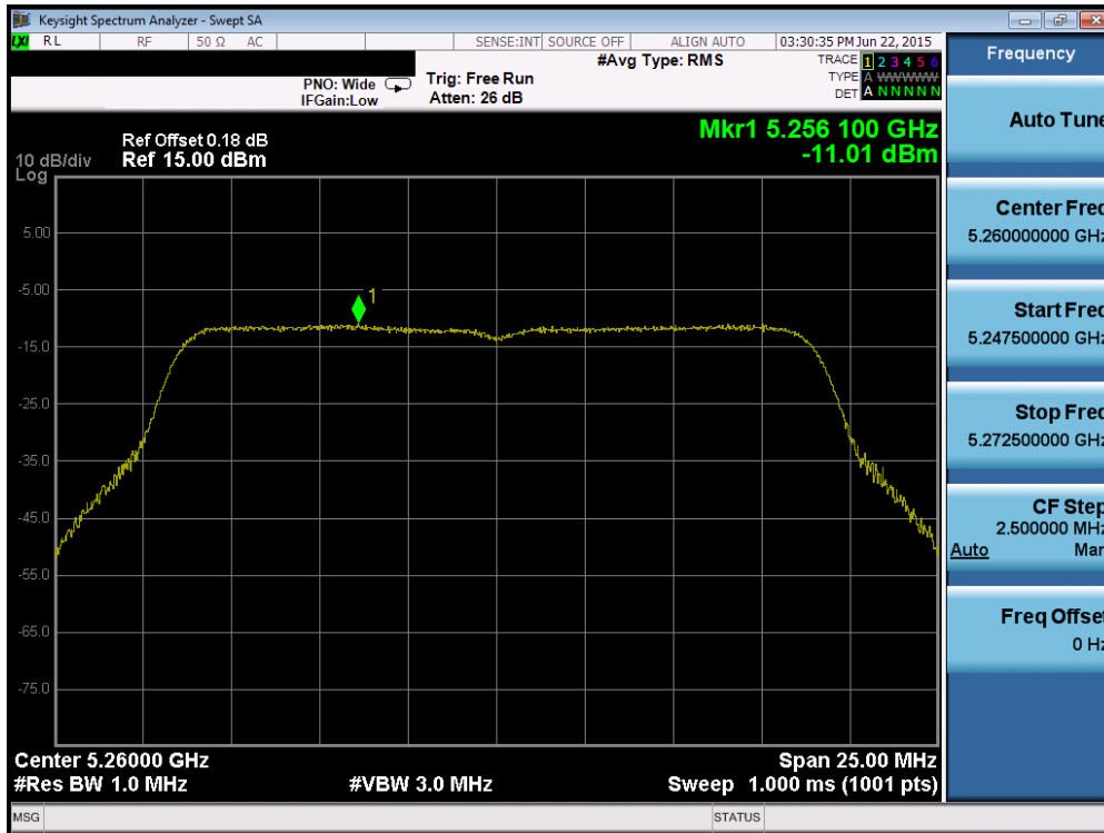
Plot 6-50. Power Spectral Density Plot (20MHz BW 802.11n (UNII Band 2A) – Ch. 52)
