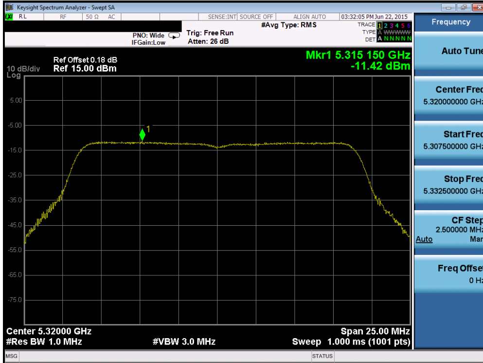
Plot 6-52. Power Spectral Density Plot (20MHz BW 802.11n (UNII Band 2A) – Ch. 64)
