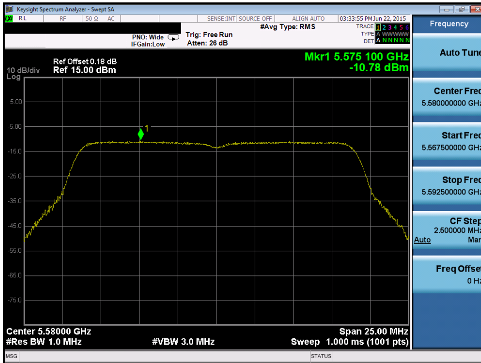
Plot 6-60. Power Spectral Density Plot (20MHz BW 802.11n (UNII Band 2C) – Ch. 116)
