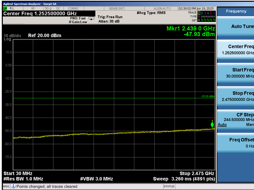
Plot 6-85. Conducted Spurious Plot (Band 7 – 20.0MHz QPSK – RB Size 1, RB Offset 0– Low Channel)
