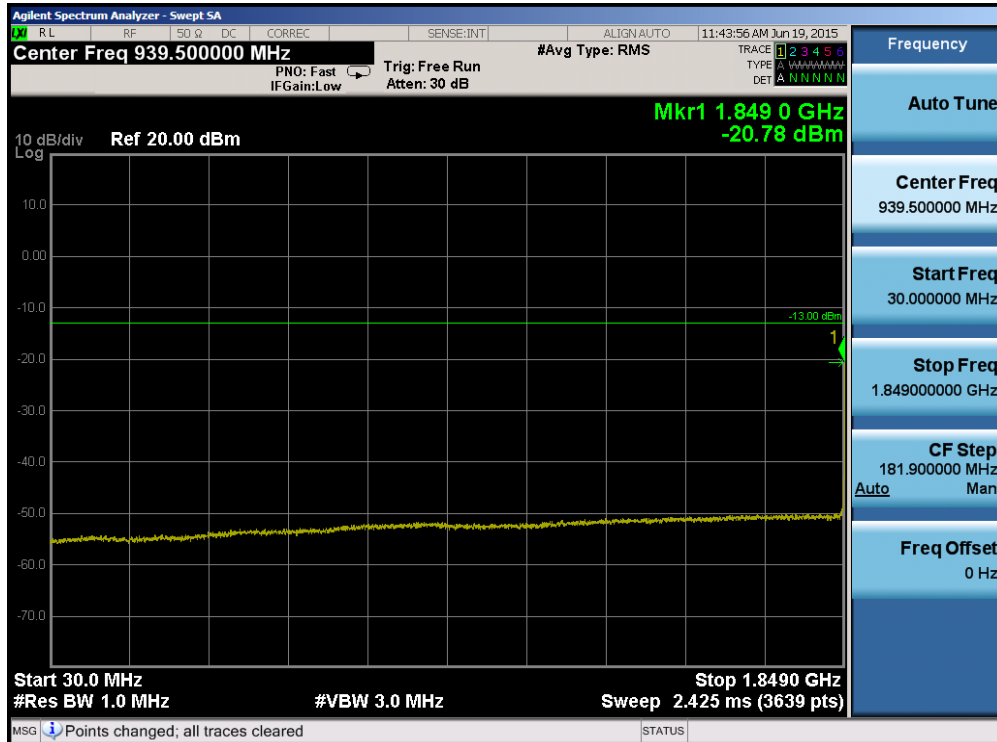
Plot 6-76. Conducted Spurious Plot (Band 2 – 1.4MHz QPSK – RB Size 1, RB Offset 0 – Low Channel)
