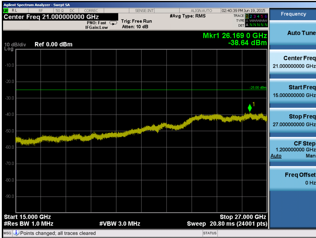
Plot 6-93. Conducted Spurious Plot (Band 7 – 20.0MHz QPSK – RB Size 1, RB Offset 0 – High Channel)
