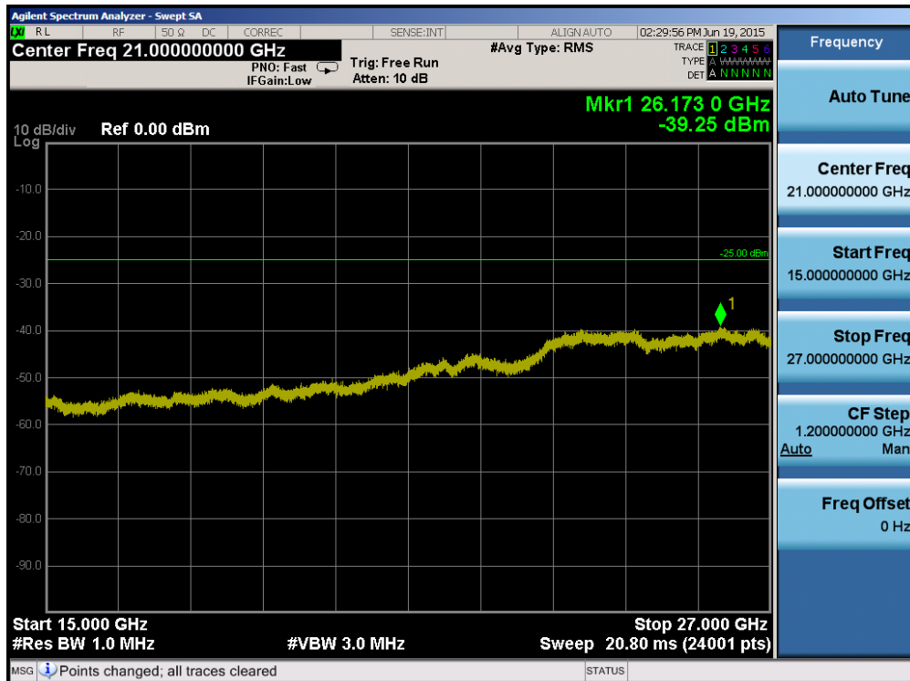
Plot 6-90. Conducted Spurious Plot (Band 7 – 20.0MHz QPSK – RB Size 1, RB Offset 0 – Mid Channel)
