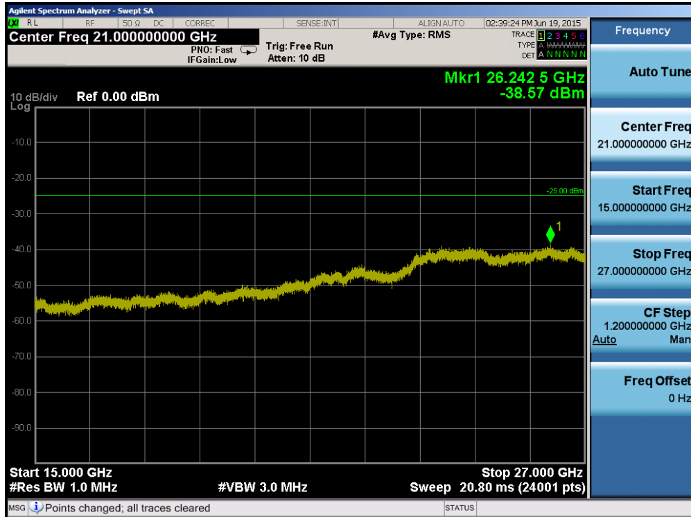
Plot 6-87. Conducted Spurious Plot (Band 7 – 20.0MHz QPSK – RB Size 1, RB Offset 0 – Low Channel)
