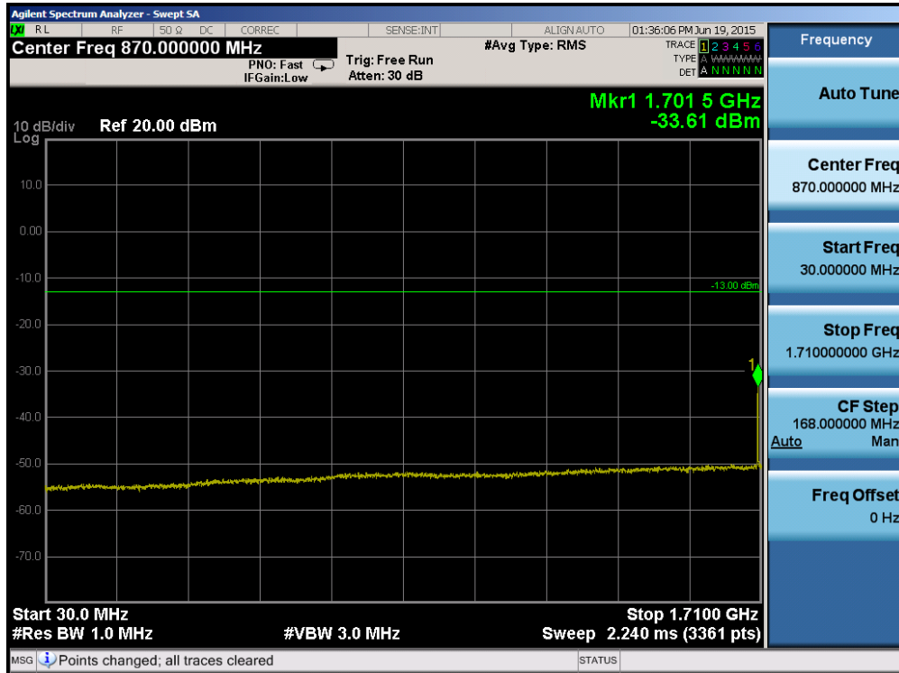
Plot 6-73. Conducted Spurious Plot (Band 4 – 20.0MHz QPSK – RB Size 1, RB Offset 0 – High Channel)
