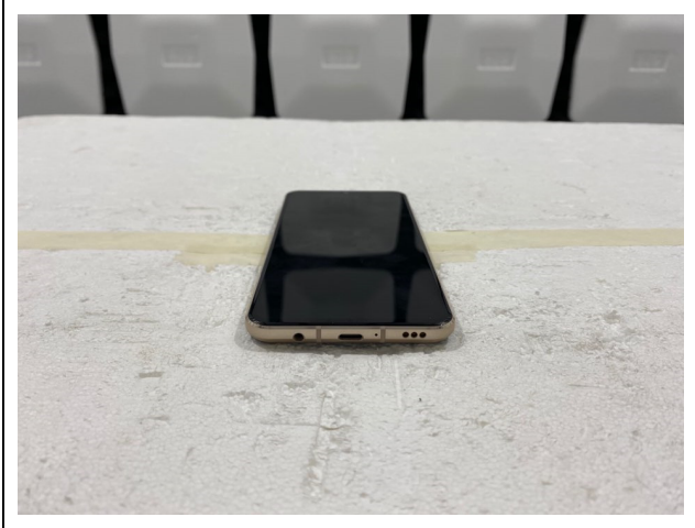
EUT Position: Y-axis
