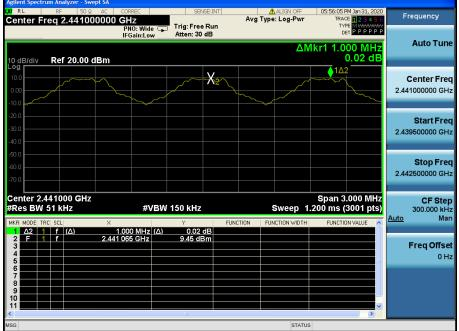
Carrier Frequency Separation (AFH) <u>Hopping mode : Enable & π/4DQPSK</u>
