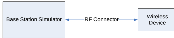
Figure 9-1 Power Measurement Setup
