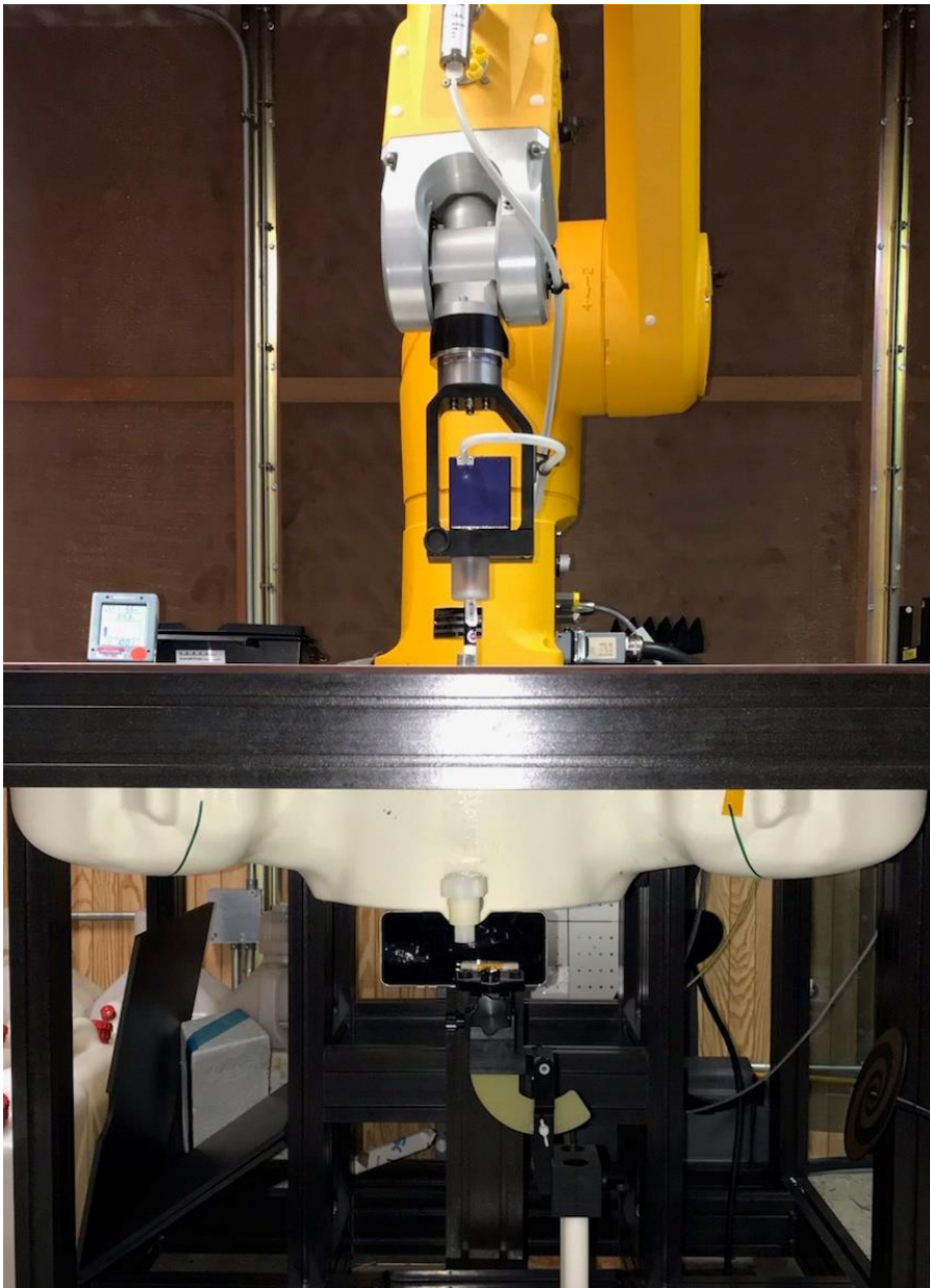
Figure 6-1 SAR measurement setup
