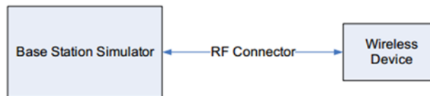
Figure 9.1 Power Measurement Setup
