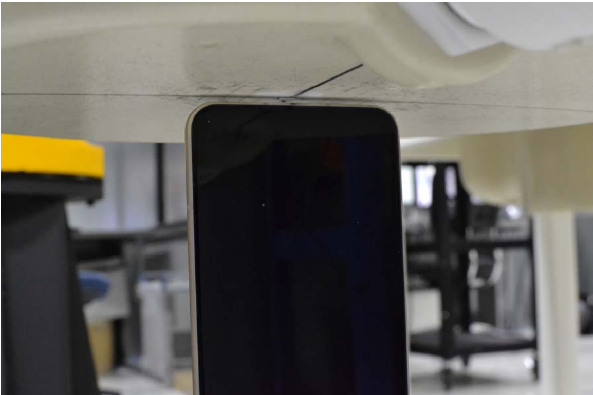
SAR Test Setup Photo 22 – Bottom Side at 3 mm
