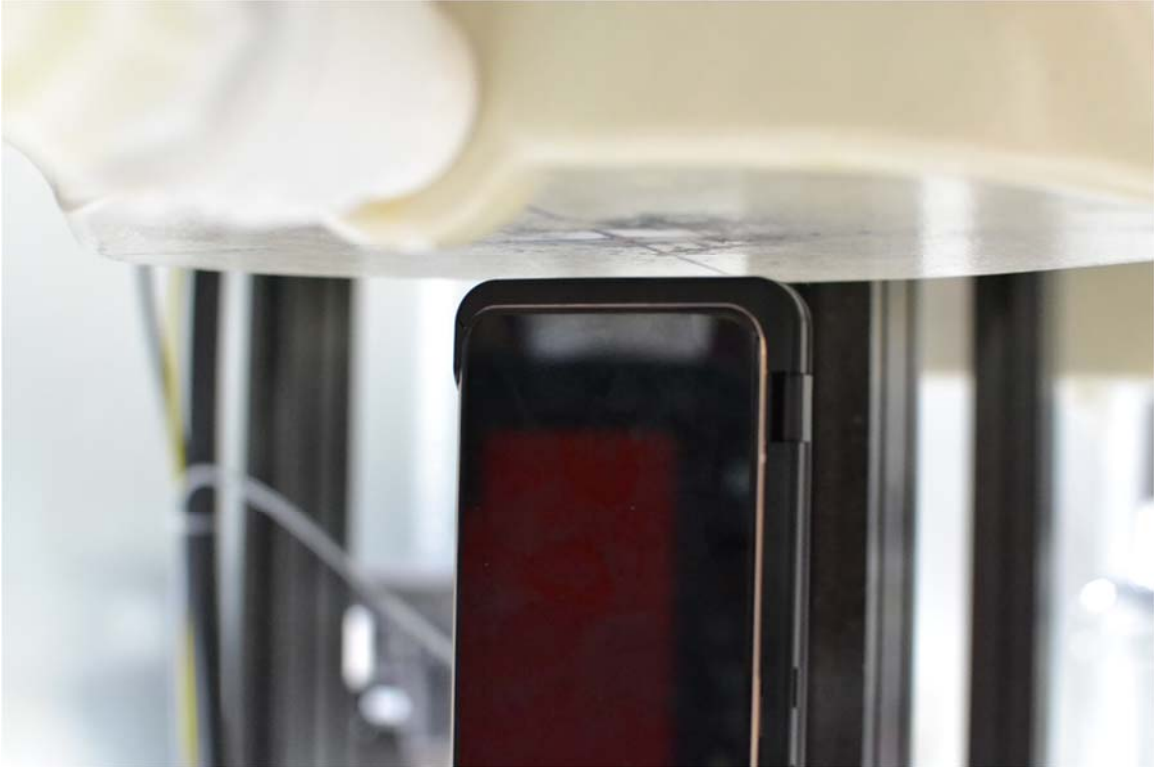
SAR Test Setup Photo 21 – Bottom Side at 10 mm with Dual Display Cover Position #3 (360 degrees)
