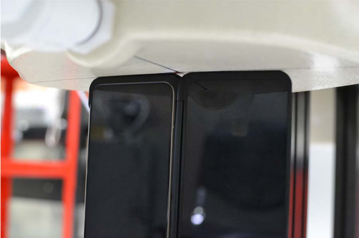
SAR Test Setup Photo 25 – Bottom Side at 0 mm with Dual Display Cover Position #2 (180 degrees)
