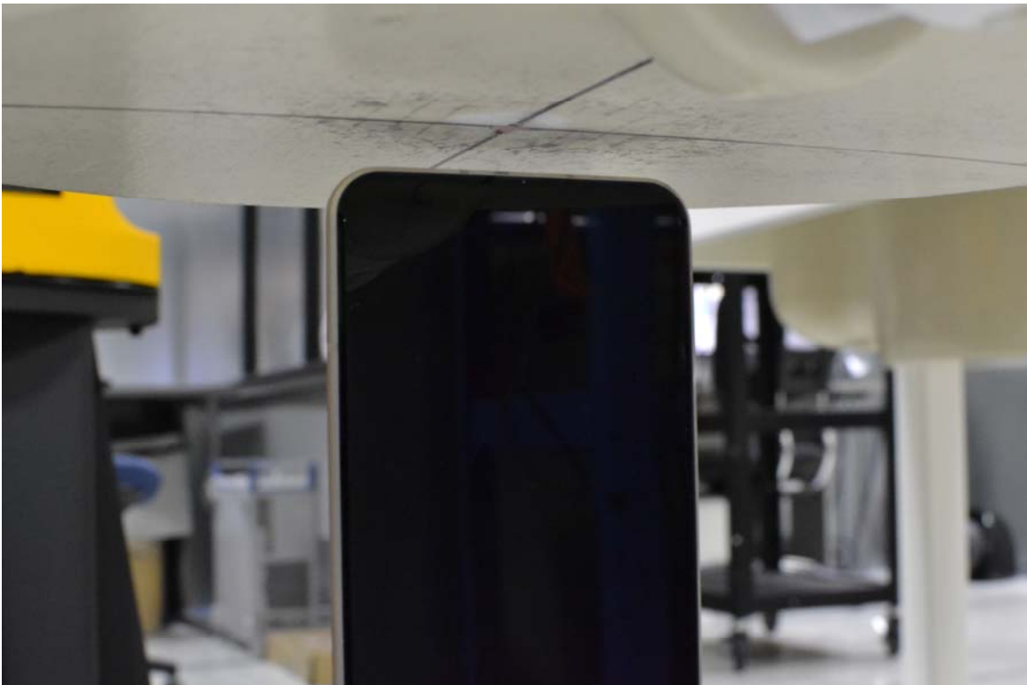
SAR Test Setup Photo 18 – Bottom Side at 10 mm
