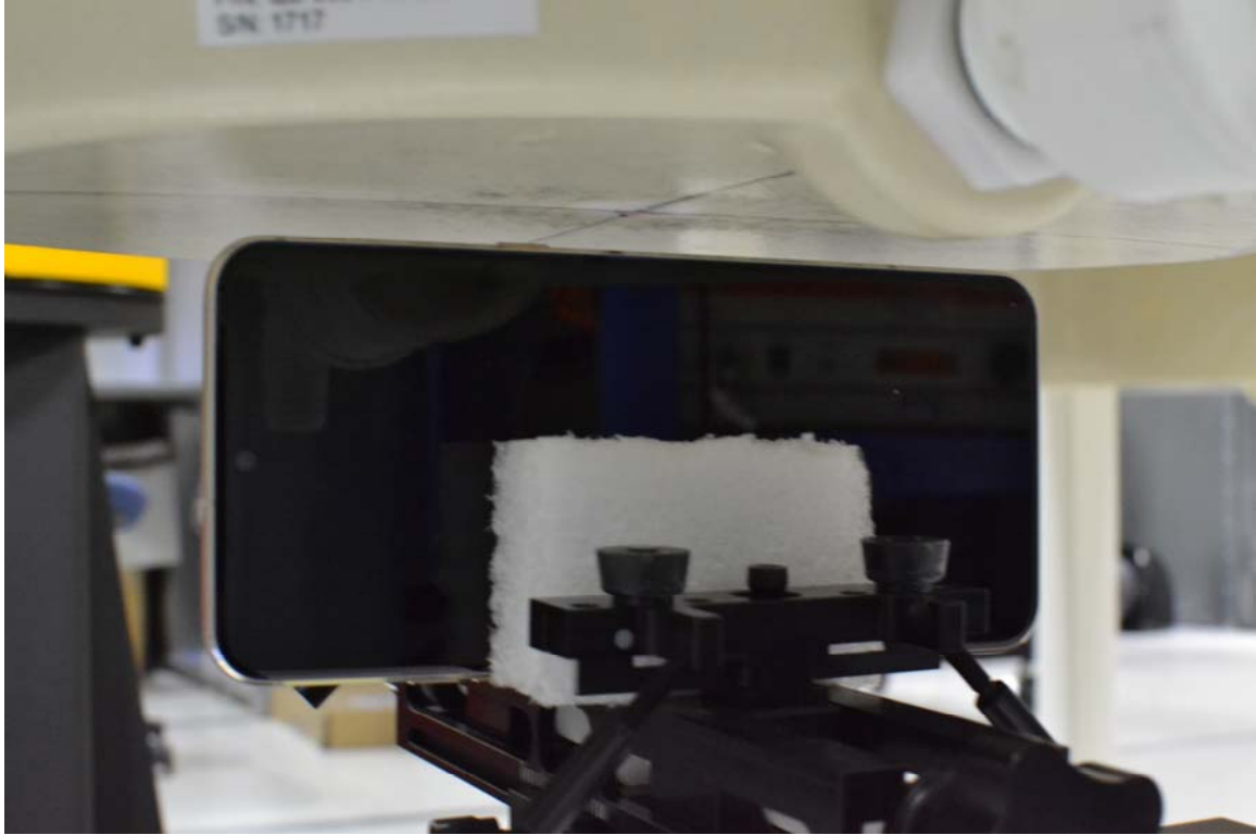
SAR Test Setup Photo 27 – Right Side at 10 mm
