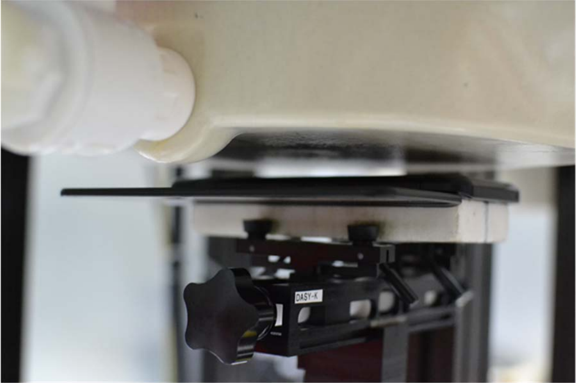
SAR Test Setup Photo 9 – Back Side at 10 mm with Dual Display Cover Position #2 (180 degrees)
