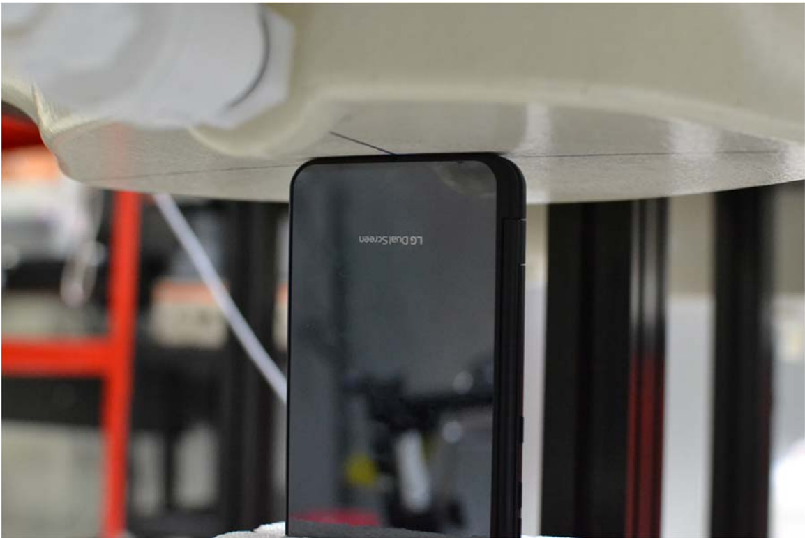
SAR Test Setup Photo 24 – Bottom Side at 0 mm with Dual Display Cover Position #1 (0 degrees)
