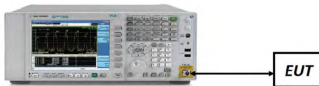
Figure 7-3. Test Instrument & Measurement Setup
