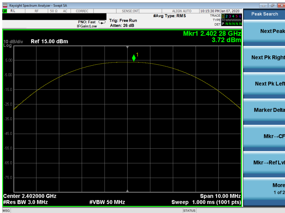
Plot 7-16. Peak Power Plot (Bluetooth (LE), 500kbps – Ch. 0)
