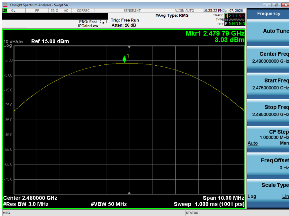
Plot 7-15. Peak Power Plot (Bluetooth (LE), 125kbps – Ch. 39)
