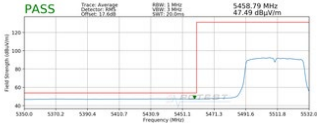
Plot 7-337. Radiated Lower Band Edge Plot MIMO (Average – UNII Band 2C)
