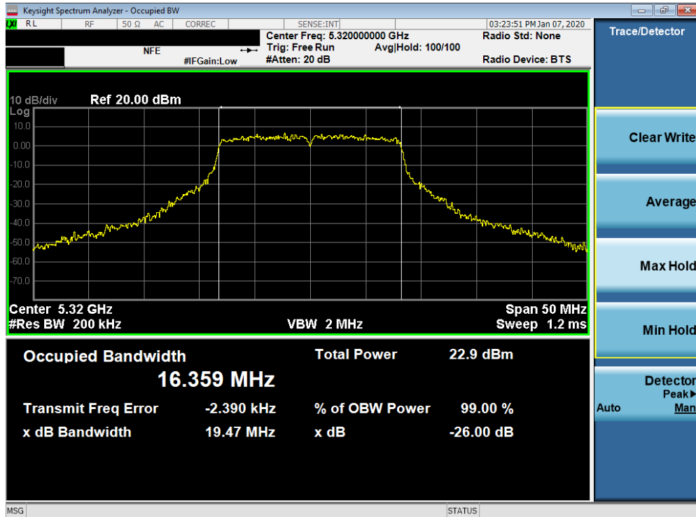
Plot 7-18. 26dB Bandwidth Plot SISO ANT1 (802.11a (UNII Band 2A) – Ch. 64)
