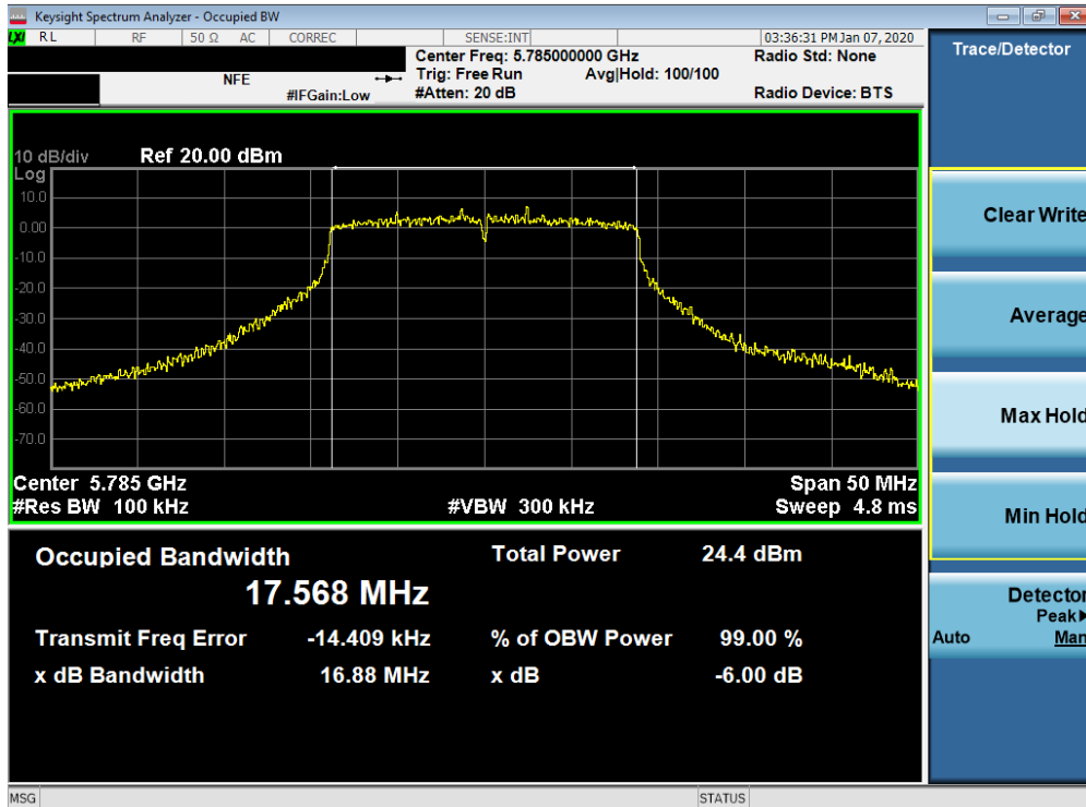
Plot 7-103. 6dB Bandwidth Plot SISO ANT1 (20MHz BW 802.11n (UNII Band 3) – Ch. 157)
