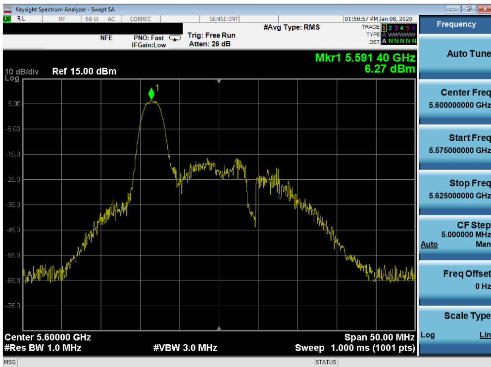
Plot 7-122. Power Spectral Density Plot SISO ANT1 (20MHz BW 802.11ax – 26 Tones (UNII Band 2C) – Ch. 120)
