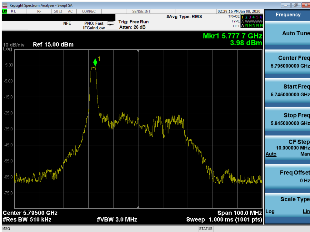
Plot 7-134. Power Spectral Density Plot SISO ANT1 (40MHz BW 802.11ax – 26 Tones (UNII Band 3) – Ch. 159)
