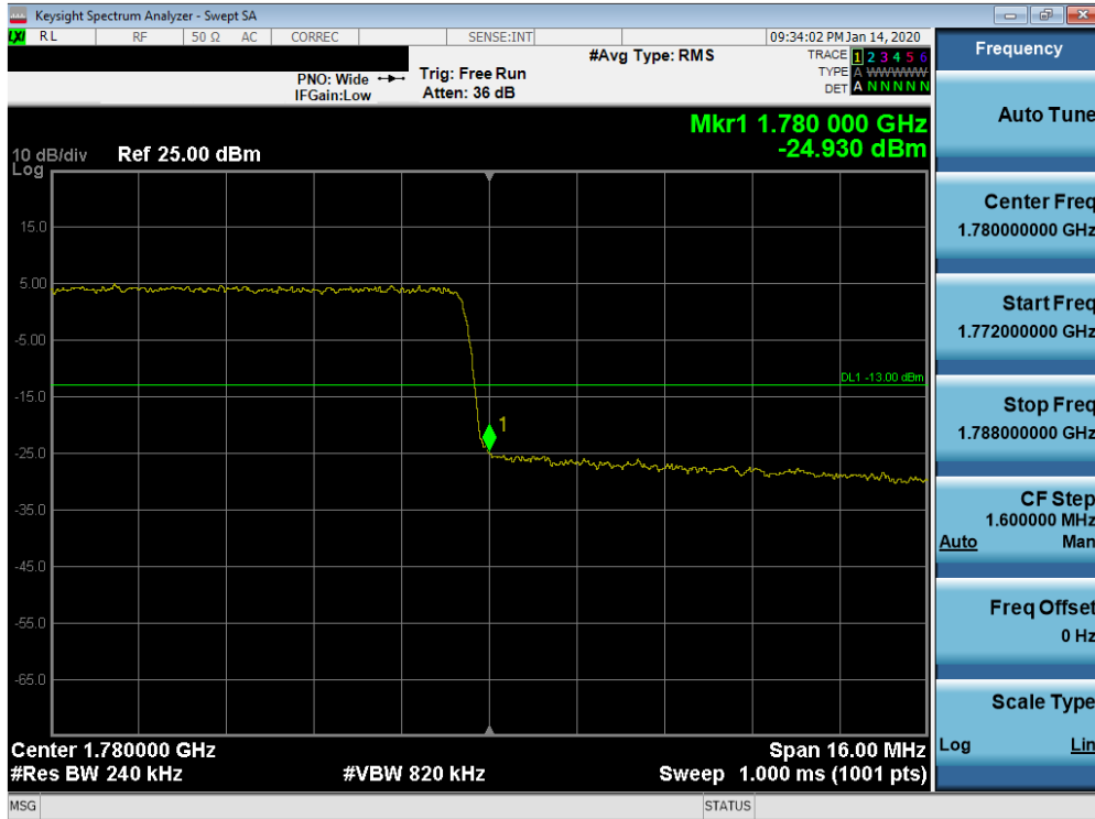
Plot 7-385. Upper Band Edge Plot (Band n66 - 20.0MHz CP-OFDM-QPSK - Full RB Configuration)
