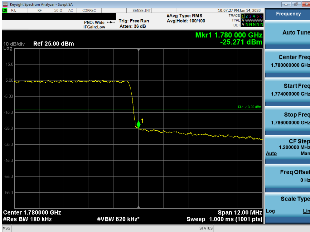
Plot 7-381. Upper Band Edge Plot (Band n66 - 15.0MHz CP-OFDM-QPSK - Full RB Configuration)
