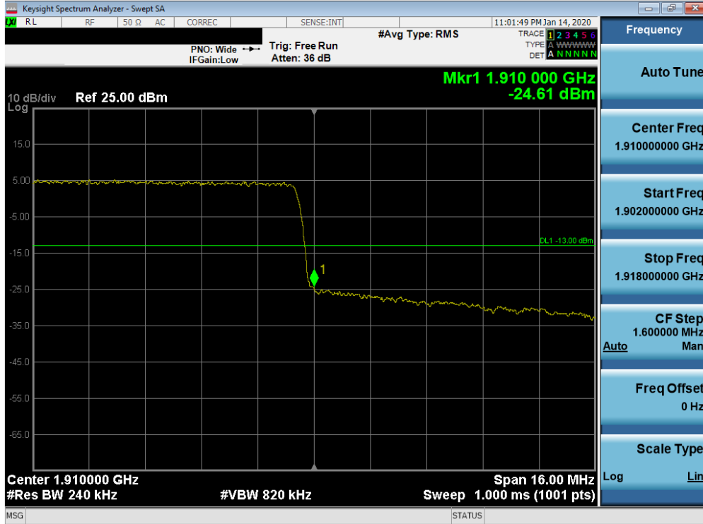
Plot 7-401. Upper Band Edge Plot (Band n2 - 20.0MHz CP-OFDM-QPSK - Full RB Configuration)
