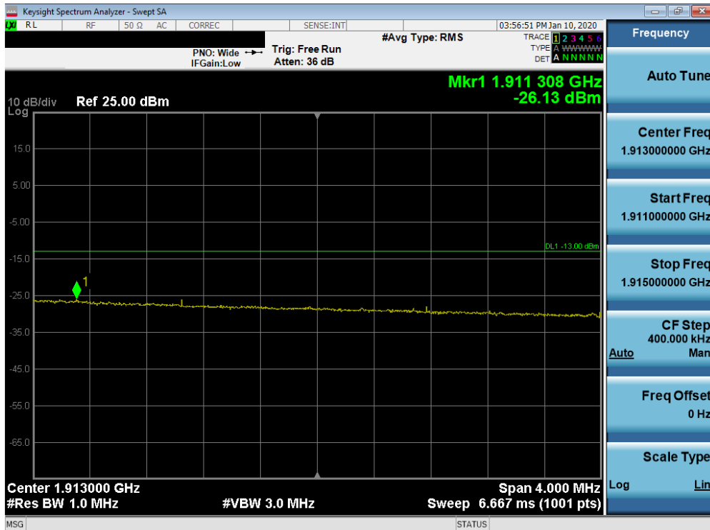
Plot 7-398. Upper Extended Band Edge Plot (Band n2 - 15.0MHz CP-OFDM-QPSK - Full RB Configuration)
