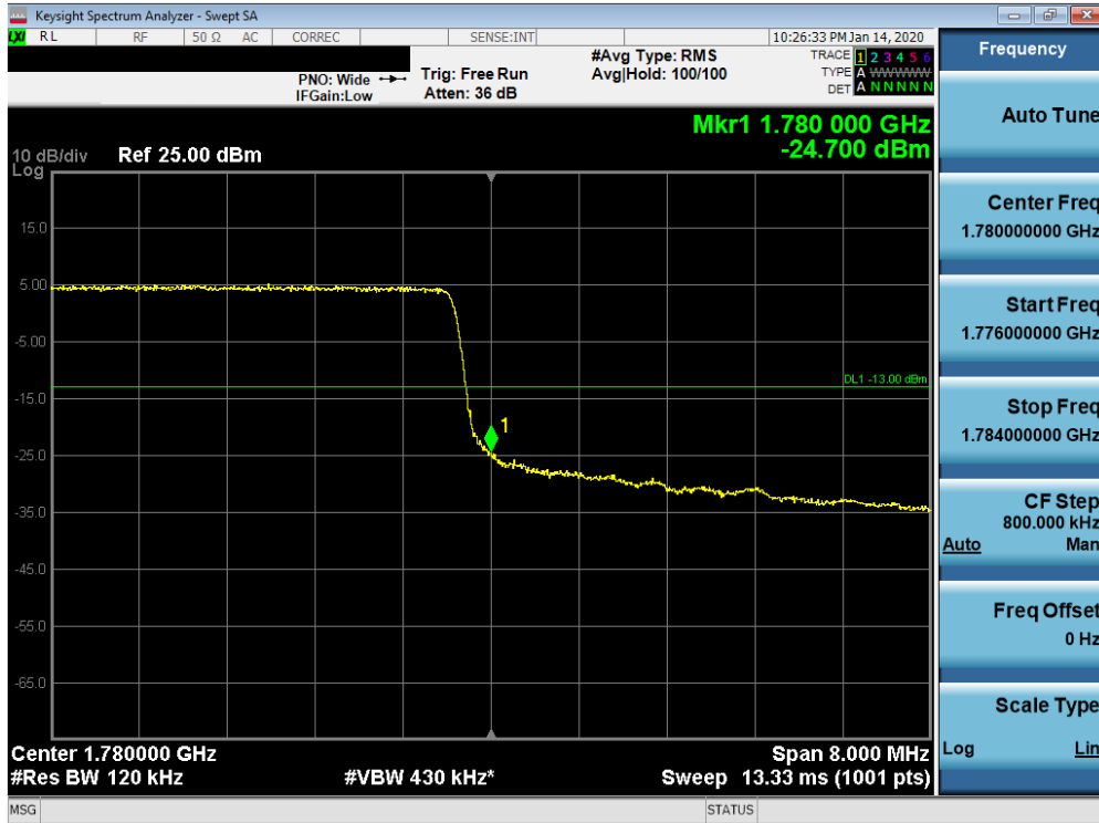
Plot 7-377. Upper Band Edge Plot (Band n66 - 10.0MHz CP-OFDM-QPSK - Full RB Configuration)
