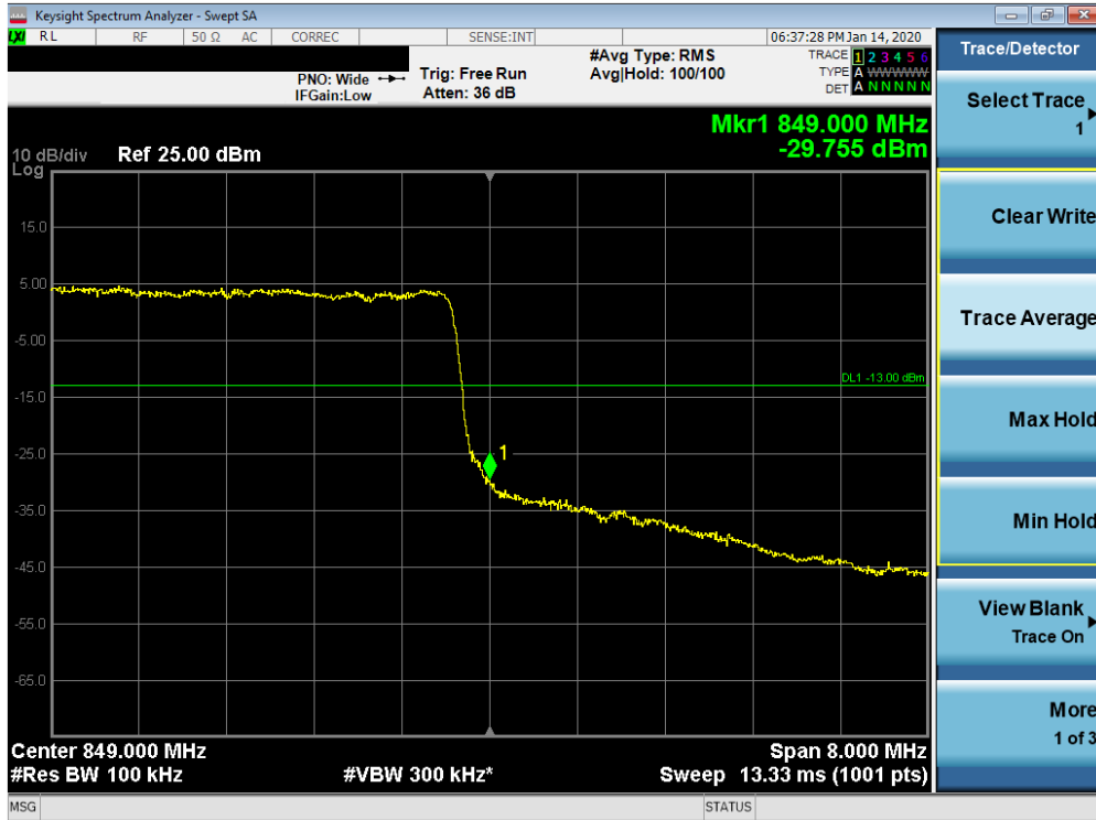
Plot 7-366. Upper Band Edge Plot (n5 - 10MHz CP-OFDM-QPSK - Full RB Configuration)
