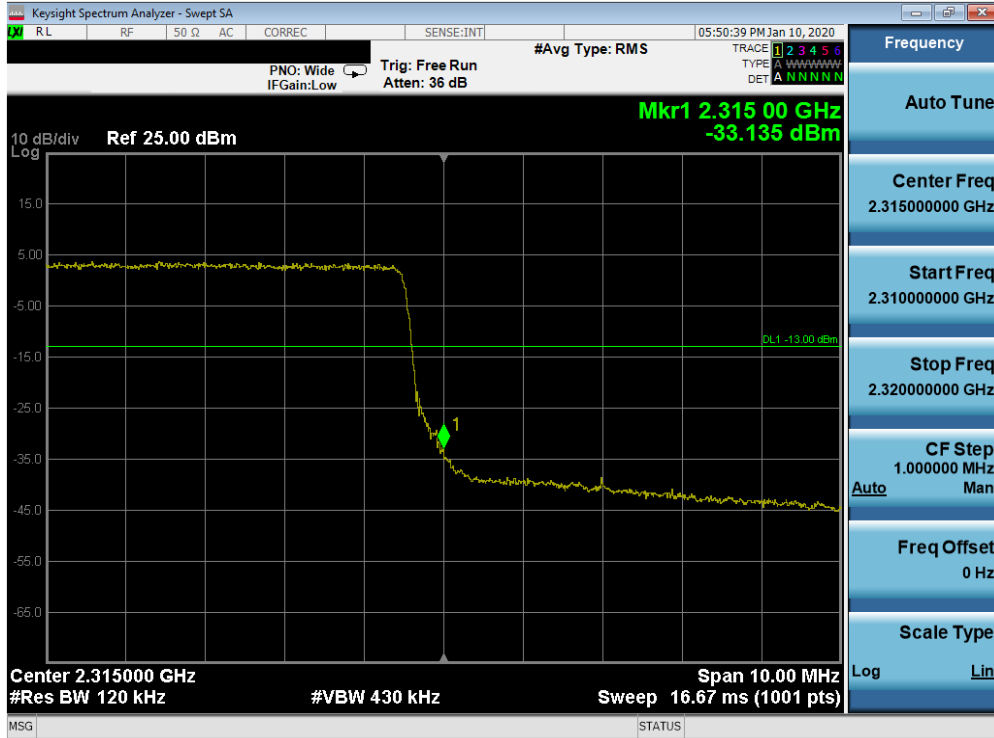
Plot 7-229. Upper Band Edge Plot (Band 30 - 10.0MHz QPSK - Full RB Configuration)
