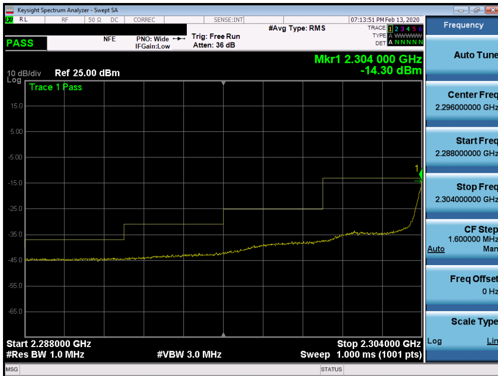
Plot 7-224. Lower Extended Band Edge Plot (Band 30 - 5.0MHz QPSK - Full RB Configuration)
