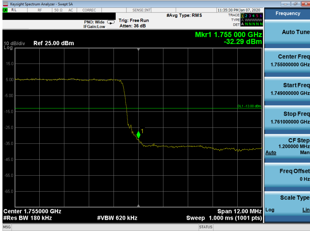
Plot 7-191. Upper Band Edge Plot (Band 4 - 15.0MHz QPSK - Full RB Configuration)
