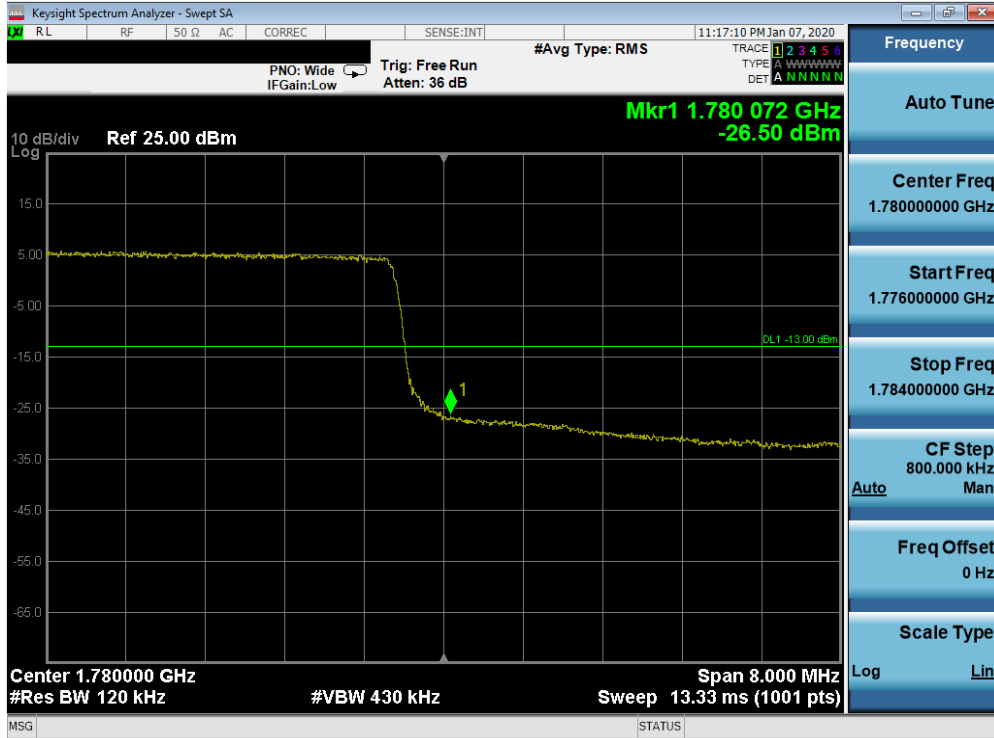
Plot 7-183. Upper Band Edge Plot (Band 66/4 - 10.0MHz QPSK - Full RB Configuration)
