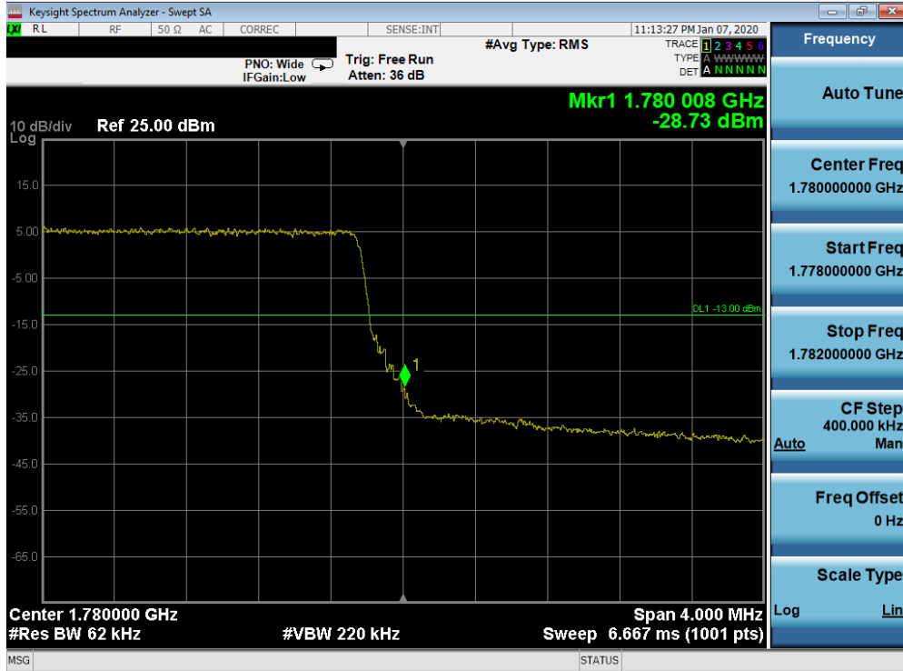
Plot 7-177. Upper Band Edge Plot (Band 66/4 - 5.0MHz QPSK - Full RB Configuration)
