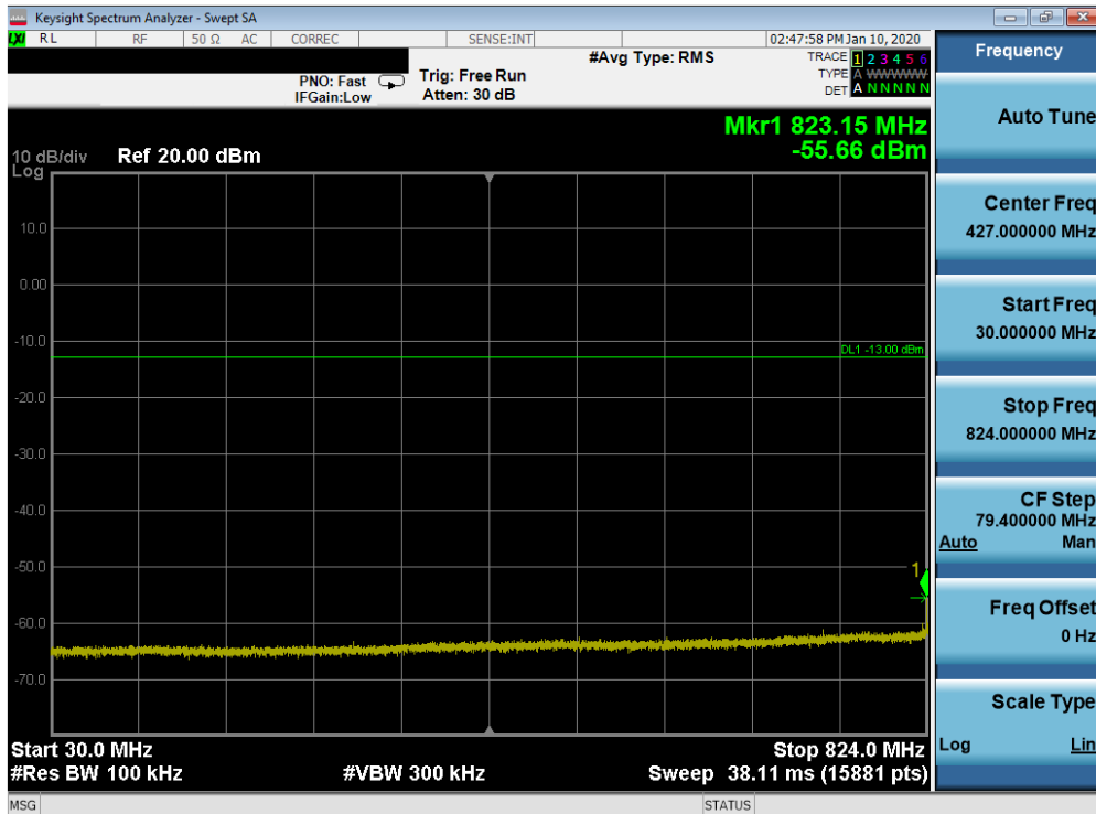
Plot 7-111. Conducted Spurious Plot (Band 5 - 10.0MHz QPSK - RB Size 1, RB Offset 0 - Mid Channel)
