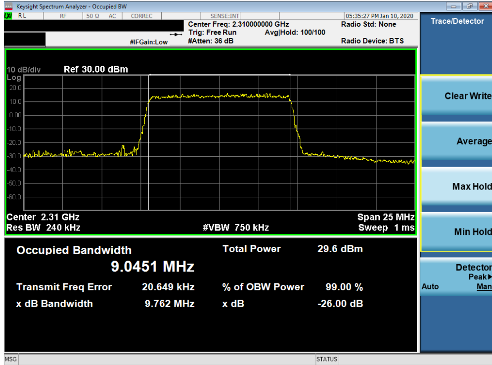
Plot 7-85. Occupied Bandwidth Plot (Band 30 - 10.0MHz QPSK - Full RB Configuration)
