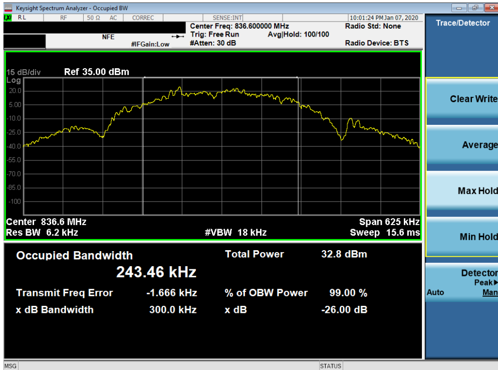
Plot 7-2. Occupied Bandwidth Plot (EDGE850 Mode)
