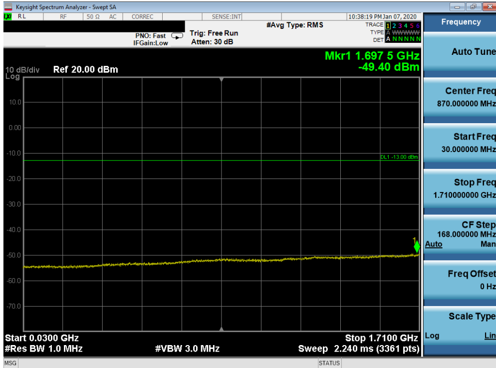
Plot 7-38. Conducted Spurious Plot (AWS WCDMA Mode - Mid Channel)
