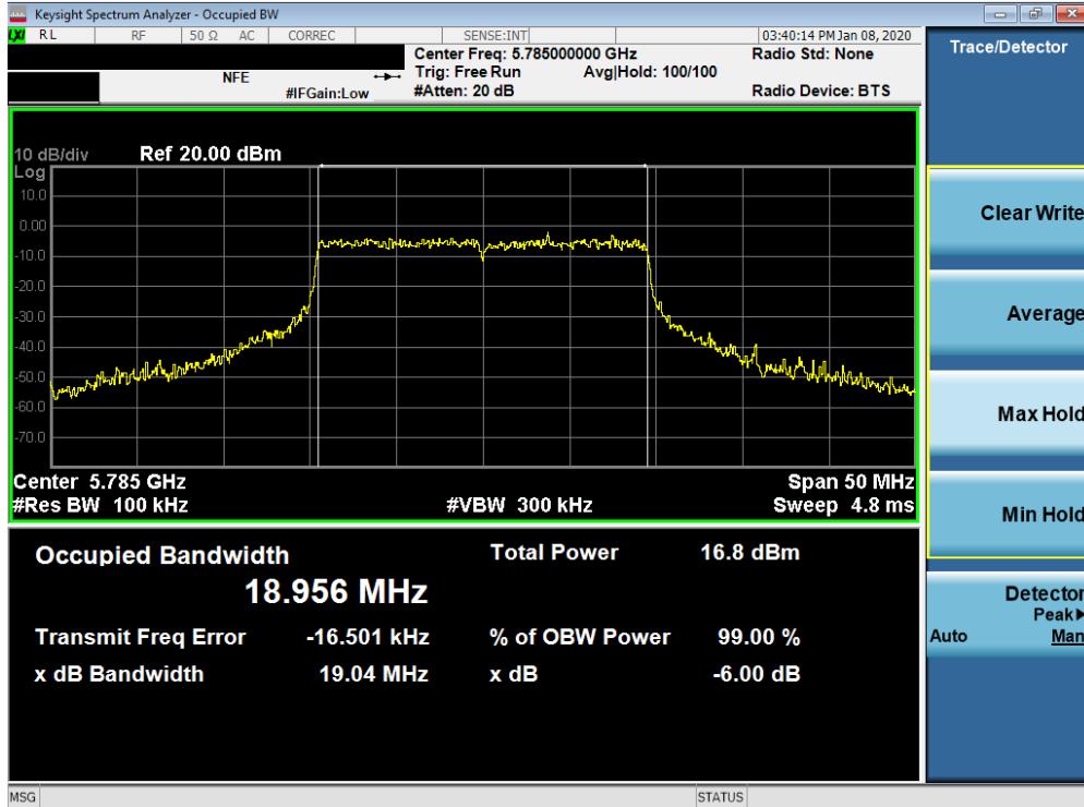
Plot 7-104. 6dB Bandwidth Plot SISO ANT2 (20MHz BW 802.11ax – Full Tones (UNII Band 3) – Ch. 157)
