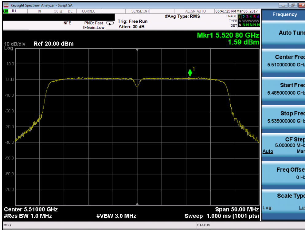
Plot 7-62. Power Spectral Density Plot (40MHz BW 802.11n (UNII Band 2C) – Ch. 102)
