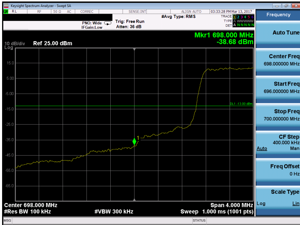
Plot 7-94. Lower Band Edge Plot (Band 12 – 1.4MHz QPSK – RB Size 6)
