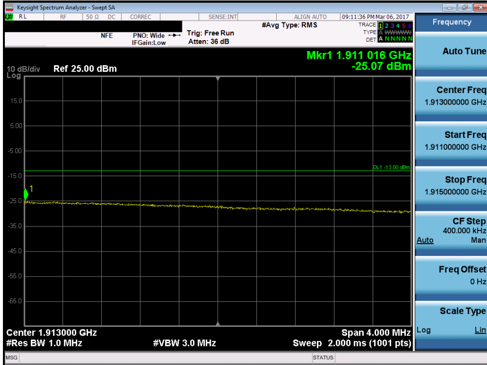
Plot 7-129. Upper Extended Band Edge Plot (Band 2 – 15.0MHz QPSK – RB Size 75)
