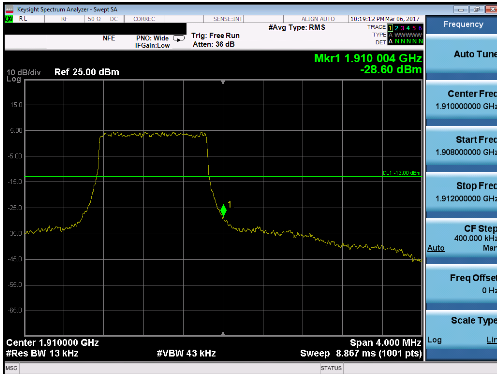
Plot 7-112. Upper Band Edge Plot (Band 2 – 1.4MHz QPSK – RB Size 6)
