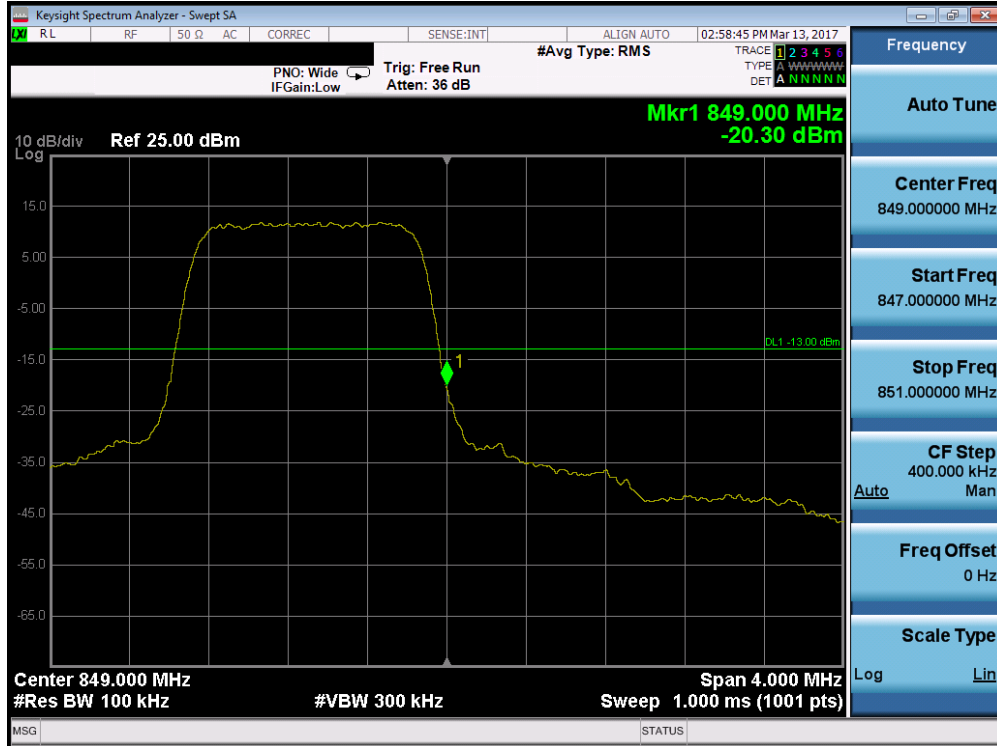
Plot 7-103. Upper Band Edge Plot (Band 5 – 1.4MHz QPSK – RB Size 6)
