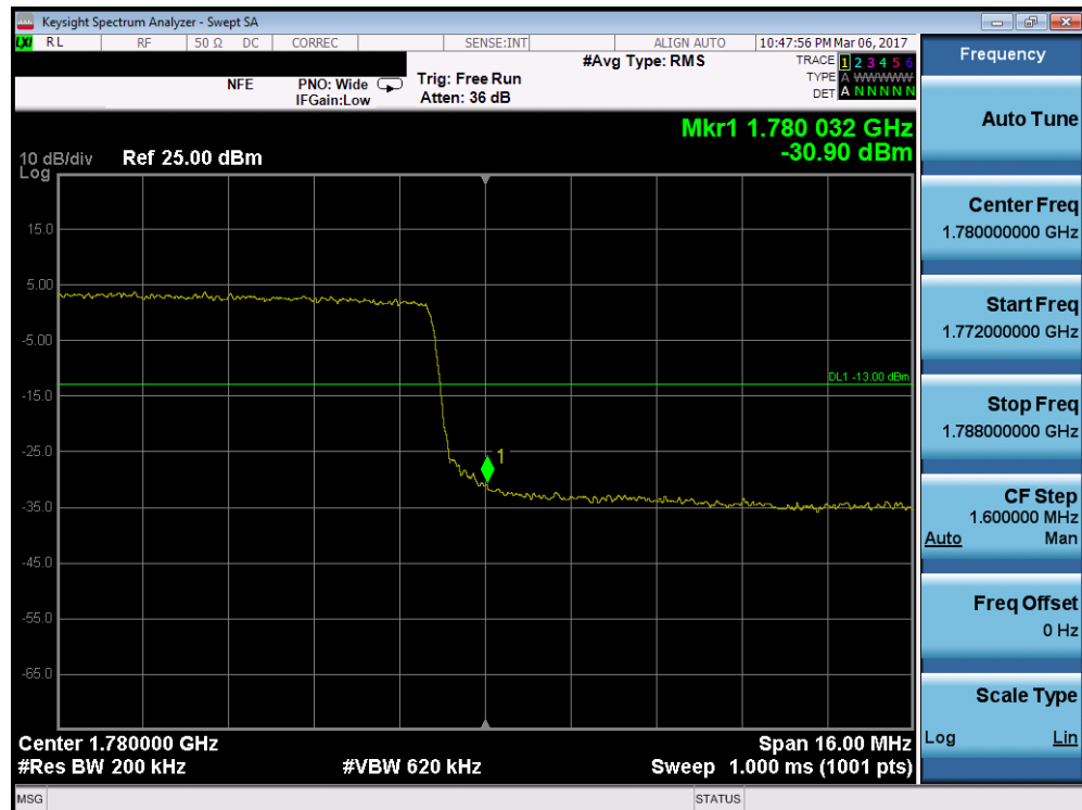
Plot 7-156. Upper Band Edge Plot (Band 66 – 20.0MHz QPSK – RB Size 100)
