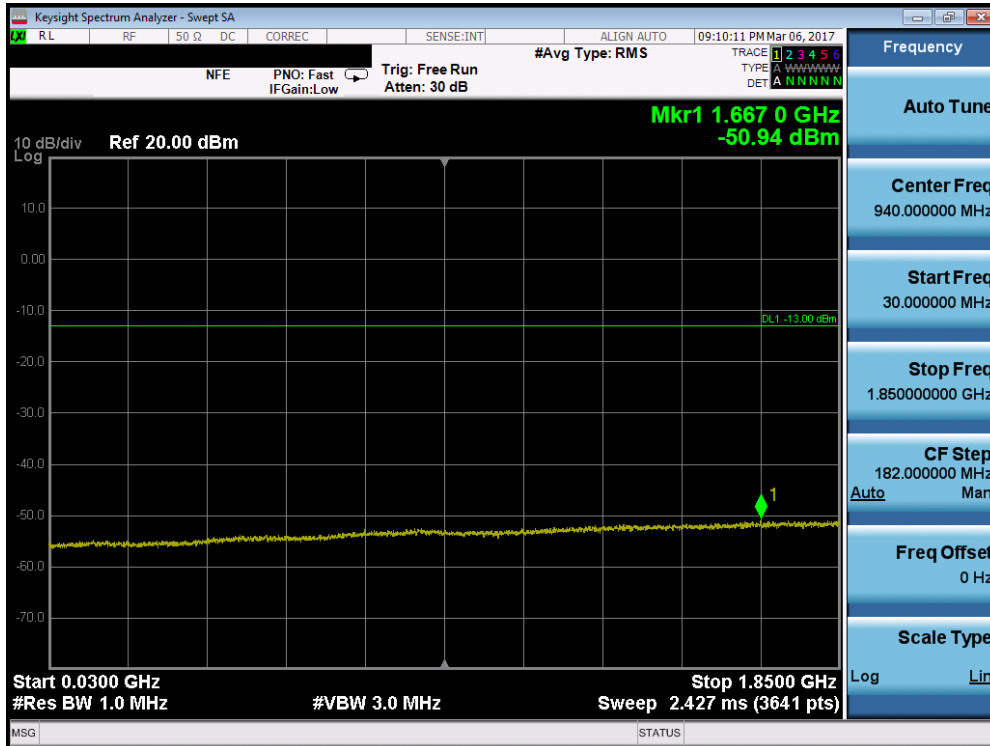
Plot 7-73. Conducted Spurious Plot (Band 2 – 15MHz QPSK – RB Size 1, RB Offset 0 – High Channel)
