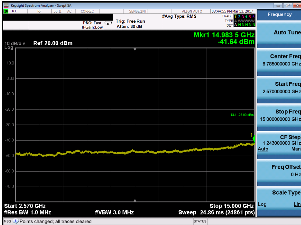
Plot 7-86. Conducted Spurious Plot (Band 7 – 10.0MHz QPSK – RB Size 1, RB Offset 0 – Low Channel)
