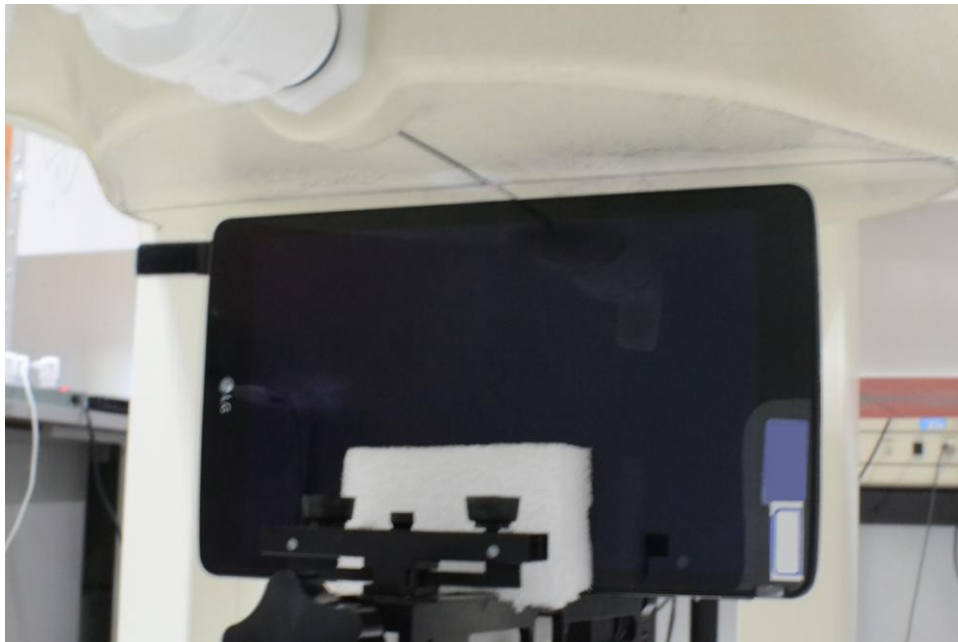
SAR Test Setup Photo 6: Left Edge at 0.5 cm
