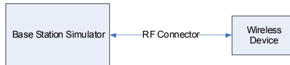
Figure 8-1 Power Measurement Setup
