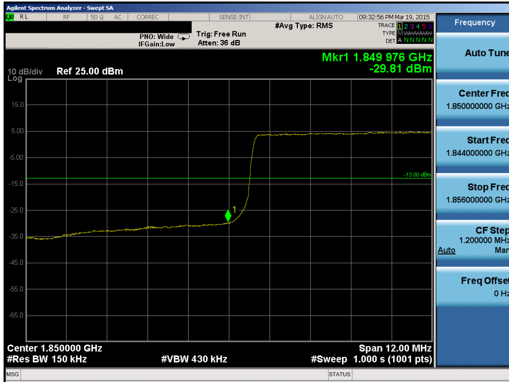
Plot 6-116. Lower Band Edge Plot (Band 2 – 15.0MHz QPSK – RB Size 75)
