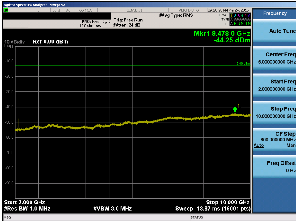
Plot 6-38. Conducted Spurious Plot (Band 12 – 3.0MHz QPSK – RB Size 1, RB Offset 0 – Mid Channel)
