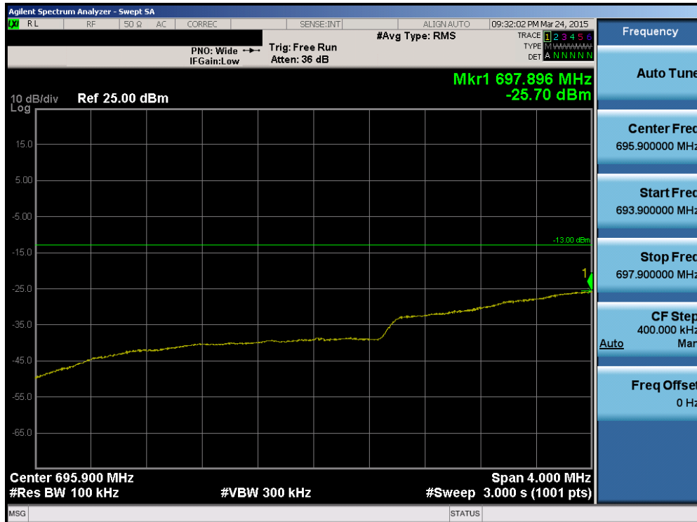
Plot 6-65. Lower Extended Band Edge Plot (Band 12 – 3.0MHz QPSK – RB Size 15)
