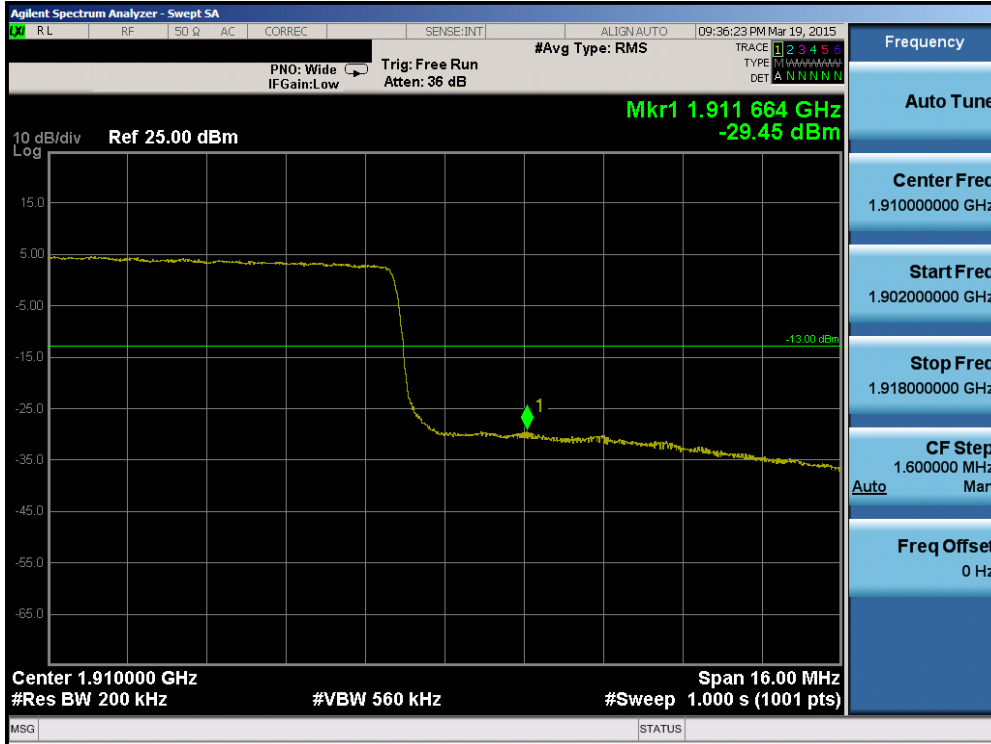
Plot 6-122. Upper Band Edge Plot (Band 2 – 20.0MHz QPSK – RB Size 100)
