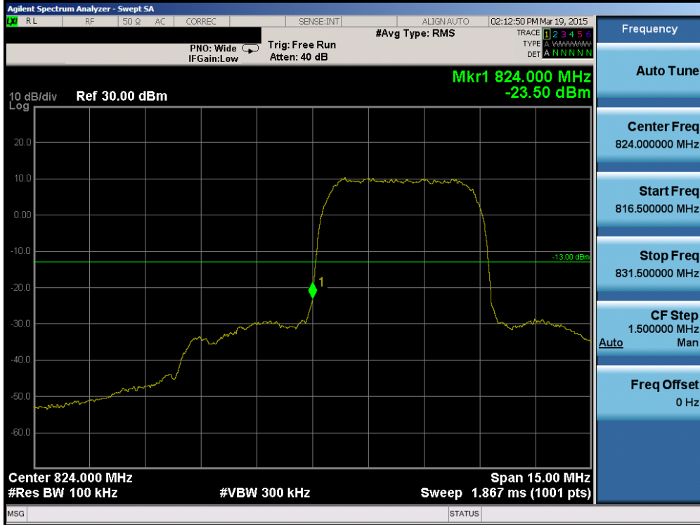
Plot 6-31. Band Edge Plot (Cellular WCDMA Mode – Ch. 4132)
