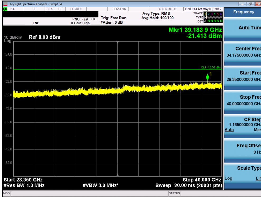
Plot 7-73. Vertical Radiated Spurious Plot 28.5-40 GHz (QTM0 1CC-100MHz Bandwidth QPSK Mid Channel)
