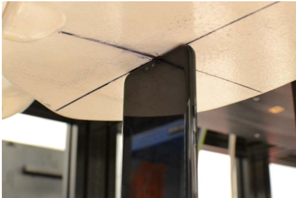
SAR Test Setup Photo 12 – Top Side at 0 mm
