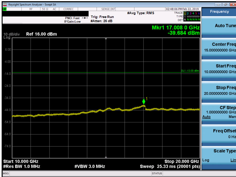
Plot 7-69. Conducted Spurious Plot (Band 66/4 - 20.0MHz QPSK - RB Size 1, RB Offset 0 - Low Channel)
