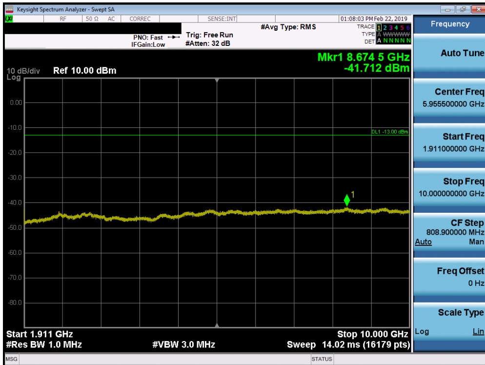
Plot 7-83. Conducted Spurious Plot (Band 2 - 20.0MHz QPSK - RB Size 1, RB Offset 0 - High Channel)
