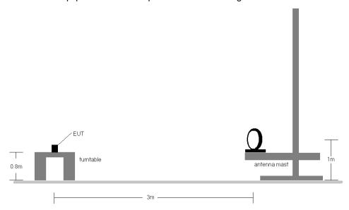
Figure 7-2. Radiated Test Setup < 30MHz
