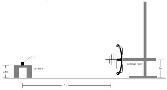
Figure 7-3. Radiated Test Setup > 30MHz
