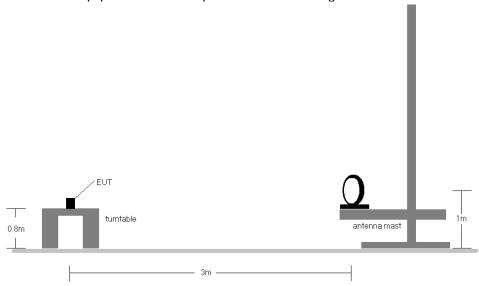
Figure 7-1. Radiated Test Setup
