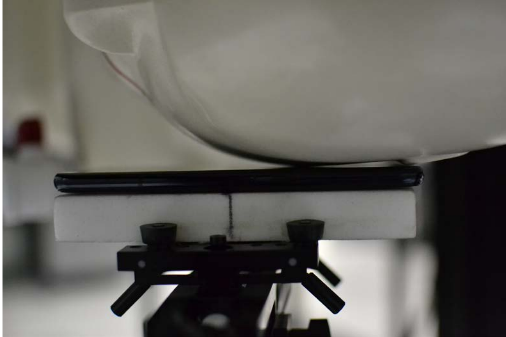
SAR Test Setup Photo 3 – Left Cheek
