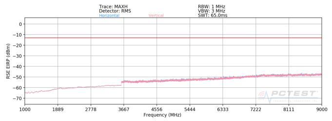
Plot 7-2. Radiated Spurious Plot above 1GHz (CDMA, Pt. 90)
