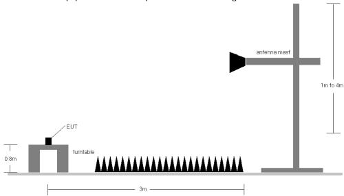
Figure 7-2. Test Instrument & Measurement Setup
