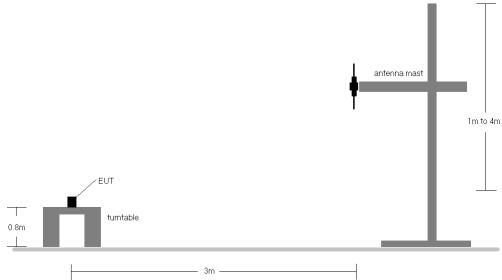
Figure 7-1. Radiated Test Setup <1GHz
