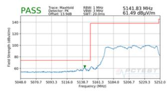
Plot 7-98. Radiated Lower Band Edge Plot MIMO (Peak – UNII Band 1)
