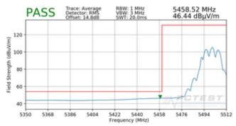
Plot 7-74. Radiated Lower Band Edge Plot CDD (Average – UNII Band 2C)
