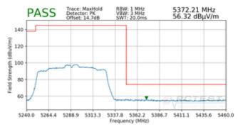
Plot 7-42. Radiated Band Edge Plot SISO ANT1 (Peak – WCP)
