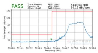
Plot 7-80. Radiated Lower Band Edge Plot MIMO (Peak – UNII Band 1)
