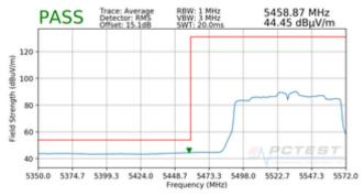
Plot 7-65. Radiated Lower Band Edge Plot SISO ANT2 (Average - UNII Band 2C)
