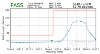
Plot 7-17. Radiated Lower Band Edge Plot SISO ANT1 (Peak - UNII Band 1)
