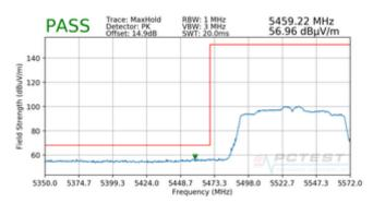
Plot 7-39. Radiated Lower Band Edge Plot SISO ANT1 (Peak – UNII Band 2C)
