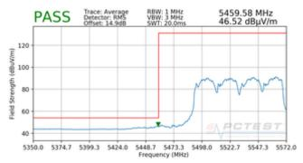
Plot 7-101. Radiated Lower Band Edge Plot MIMO (Average - UNII Band 2C)
