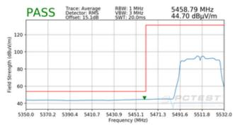
Plot 7-56. Radiated Lower Band Edge Plot SISO ANT2 (Average – UNII Band 2C)
