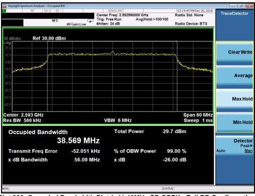
Plot 303. Occupied Bandwidth Plot (n41 40MHz CP-QPSK - Full RB Configuration)
