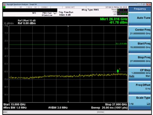
Plot 323. Conducted Spurious Plot (n41 - 40MHz CP-QPSK - RB Size 53, RB Offset 26 - High Channel)
