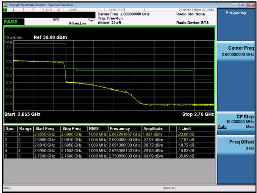
Plot 325. Upper Band Edge Plot (n41 - 60MHz CP-QPSK - Full RB Configuration)
