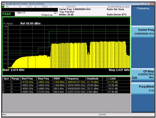
Table 7-290. Lower ACP Plot (Band 41 QPSK – PCC:20 MHz SCC:20 MHz – Full RB)
