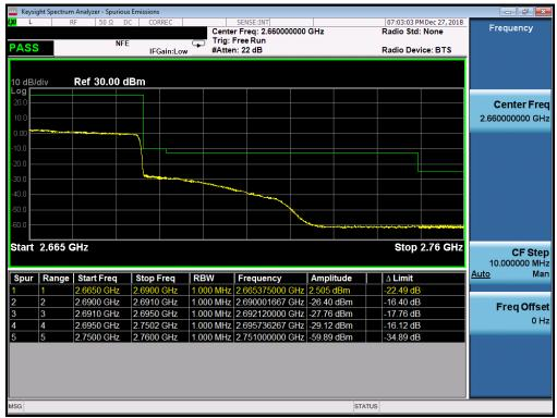
Plot 327. Upper Band Edge Plot (n41 - 60MHz CP-16QAM - Full RB Configuration)
