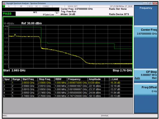
Plot 333. Upper Band Edge Plot (n41 - 40MHz CP-16QAM - Full RB Configuration)
