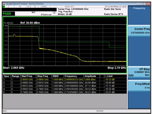
Plot 331. Upper Band Edge Plot (n41 - 40MHz CP-QPSK - Full RB Configuration)
