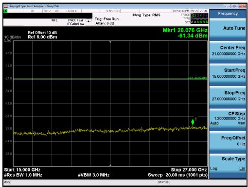
Plot 311. Conducted Spurious Plot (n41 - 60MHz CP-QPSK - RB Size 1, RB Offset 81 – Mid Channel)
