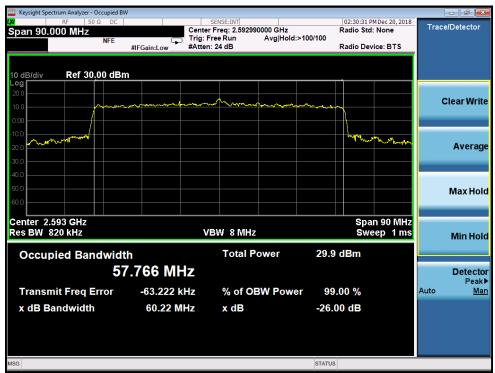
Plot 300. Occupied Bandwidth Plot (n41 60MHz CP-QPSK - Full RB Configuration)
