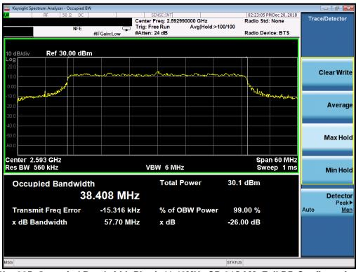
Plot 305. Occupied Bandwidth Plot (n41 40MHz CP-64QAM- Full RB Configuration)
