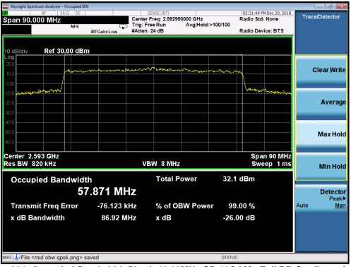
Plot 301. Occupied Bandwidth Plot (n41 60MHz CP-16QAM - Full RB Configuration)
