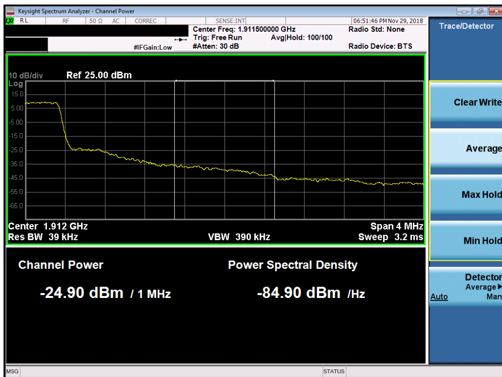
Plot 7-223. Upper Extended Band Edge Plot (Band 2 - 1.4MHz QPSK - Full RB Configuration)
