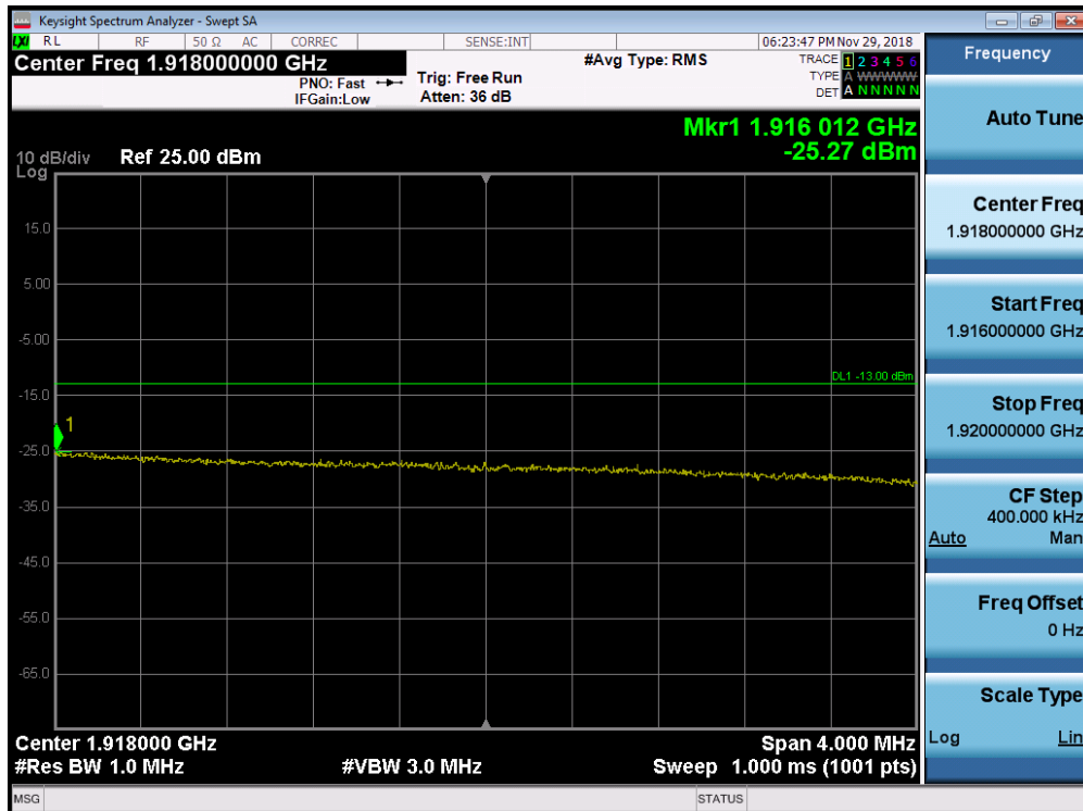
Plot 7-255. Upper Extended Band Edge Plot (Band 25 - 20.0MHz QPSK - Full RB Configuration)
