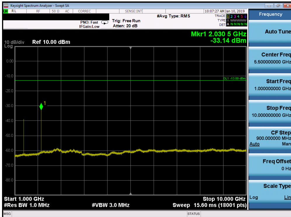
Plot 7-99. Conducted Spurious Plot (Band 71 - 10.0MHz QPSK - RB Size 1, RB Offset 0 - Mid Channel)
