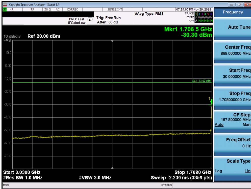
Plot 7-121. Conducted Spurious Plot (Band 66/4 - 10.0MHz QPSK - RB Size 1, RB Offset 0 - Low Channel)
