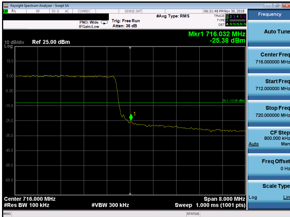
Plot 7-165. Upper Band Edge Plot (Band 12/17 - 10.0MHz QPSK - Full RB Configuration)
