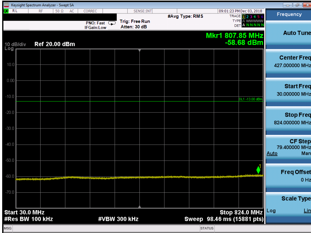
Plot 7-118. Conducted Spurious Plot (Band 26/5 - 10.0MHz QPSK - RB Size 1, RB Offset 0 - High Channel)
