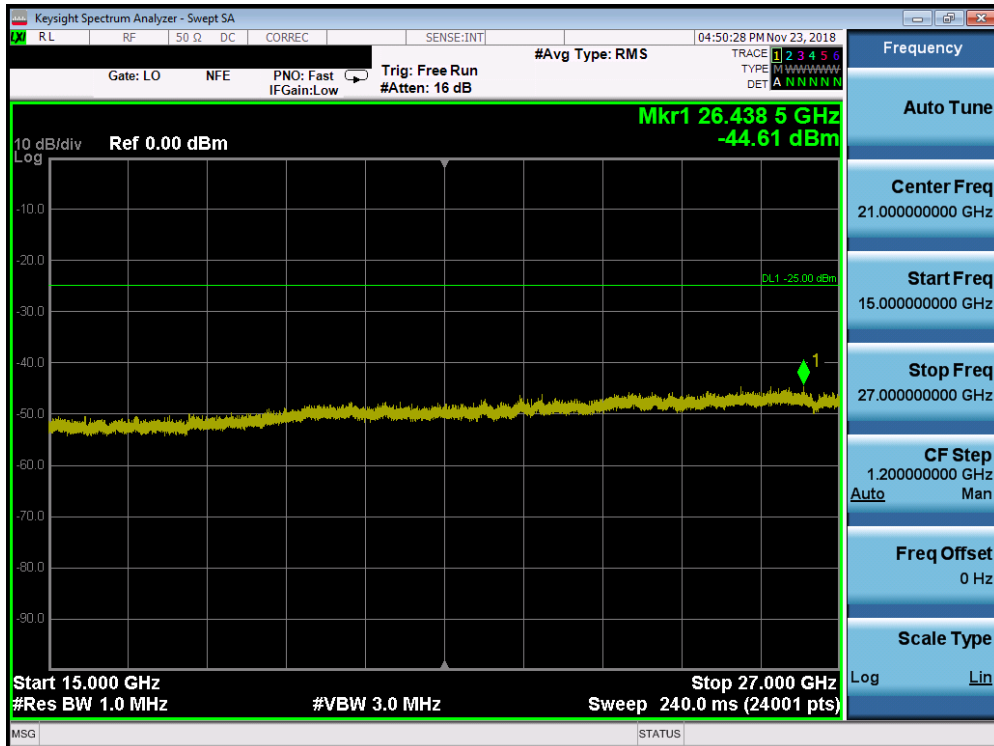
Plot 7-144. Conducted Spurious Plot (Band 41 - 10.0MHz QPSK - RB Size 1, RB Offset 0 - Mid Channel)
