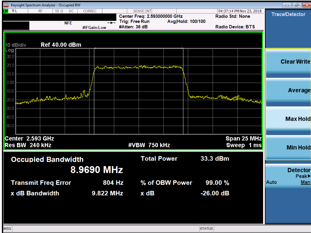
Plot 7-86. Occupied Bandwidth Plot (Band 41 (PC2) - 10.0MHz 16-QAM - Full RB Configuration)
