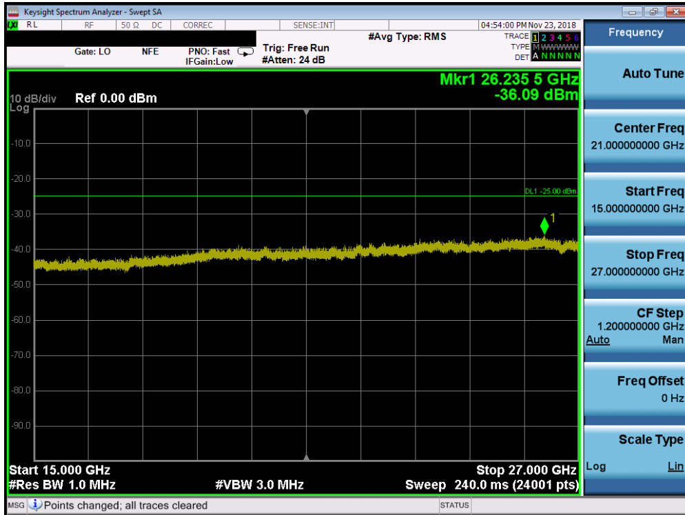
Plot 7-141. Conducted Spurious Plot (Band 41 - 10.0MHz QPSK - RB Size 1, RB Offset 0 - Low Channel)
