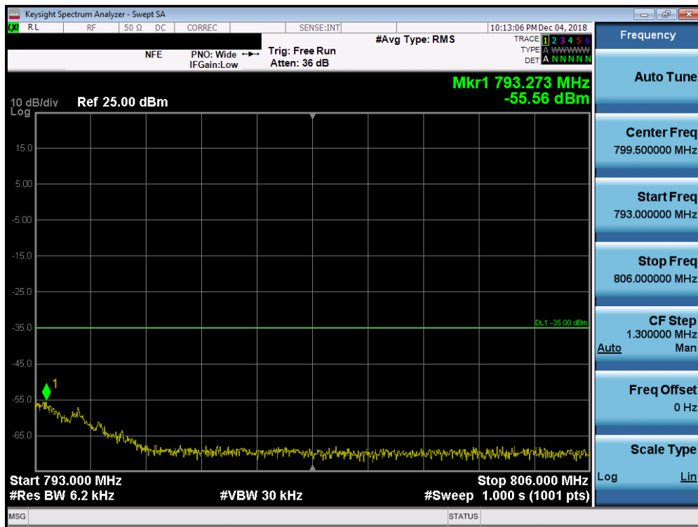
Plot 7-169. Upper Emission Mask Plot (Band 13 - 5.0MHz QPSK - Full RB Configuration)
