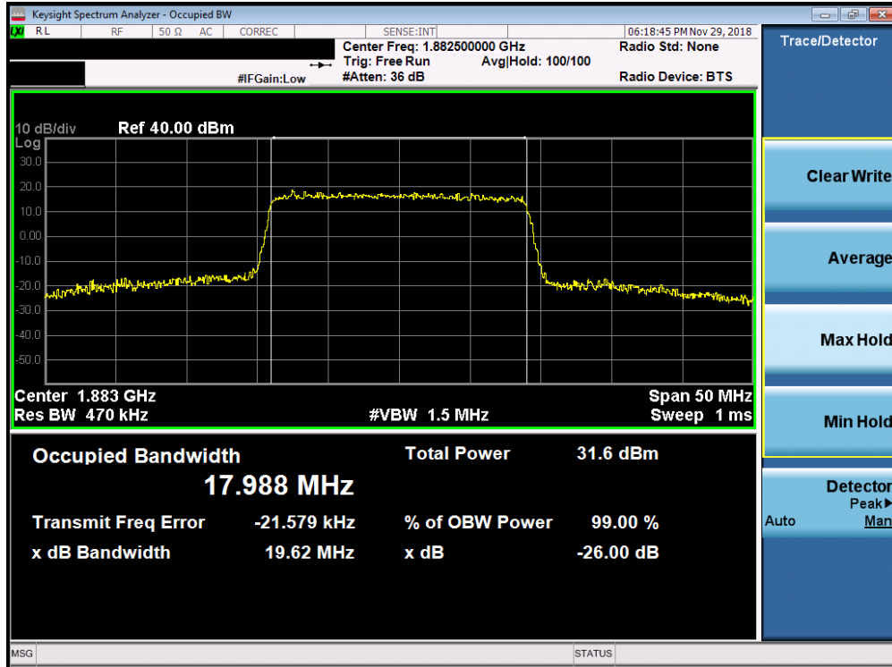
Plot 7-80. Occupied Bandwidth Plot (Band 25/2 - 20.0MHz 16-QAM - Full RB Configuration)
