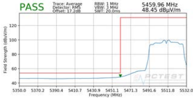
Plot 7-187. Radiated Lower Band Edge Plot SISO ANT1 (Average – UNII Band 2C)
