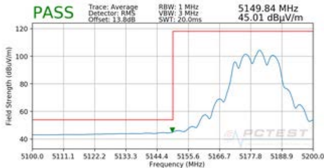
Plot 7-228. Radiated Lower Band Edge Plot CDD (Average – UNII Band 1)
