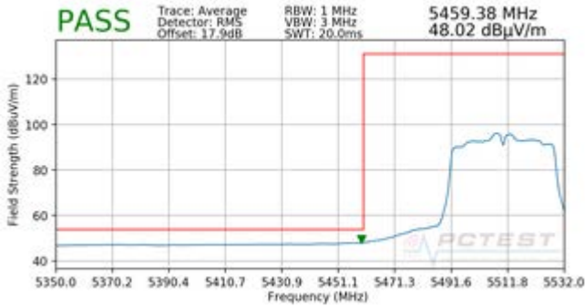
Plot 7-217. Radiated Band Edge Plot SISO ANT2 (Average – WCP)
