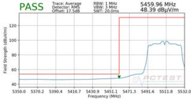
Plot 7-214. Radiated Lower Band Edge Plot SISO ANT2 (Average – UNII Band 2C)
