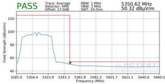
Plot 7-185. Radiated Upper Band Edge Plot SISO ANT1 (Average – UNII Band 2A)
