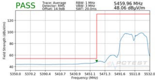
Plot 7-241. Radiated Lower Band Edge Plot MIMO (Average – UNII Band 2C)
