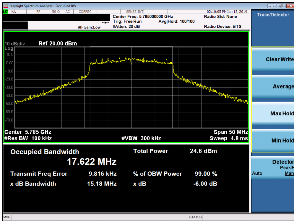
Plot 7-65. 6dB Bandwidth Plot SISO ANT1 (20MHz BW 802.11n (UNII Band 3) – Ch. 157)
