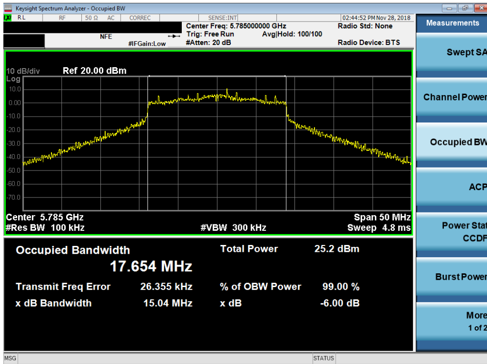
Plot 7-74. 6dB Bandwidth Plot SISO ANT2 (20MHz BW 802.11n (UNII Band 3) – Ch. 157)
