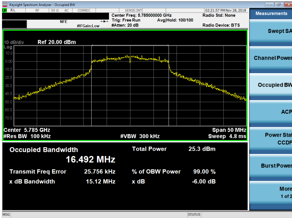
Plot 7-71. 6dB Bandwidth Plot SISO ANT2 (802.11a (UNII Band 3) – Ch. 157)
