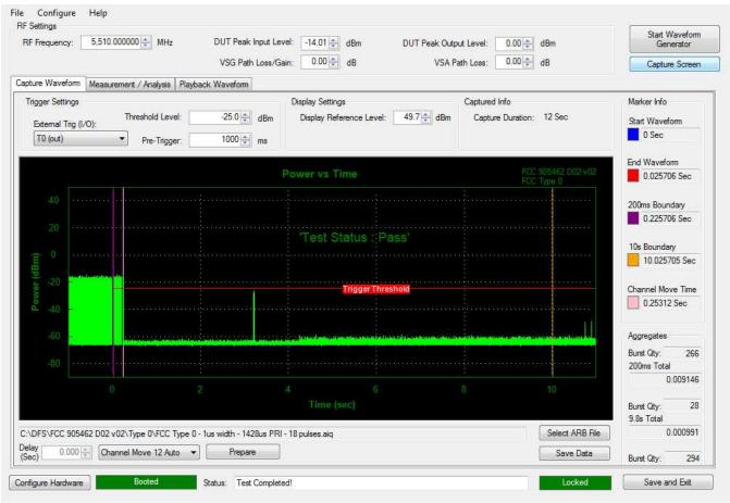
Figure 5-4. Band 2C Move Time and Aggregate Time
