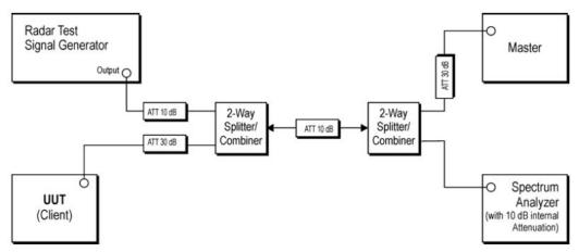
Figure 3-1. Conducted Test Setup for DFS
