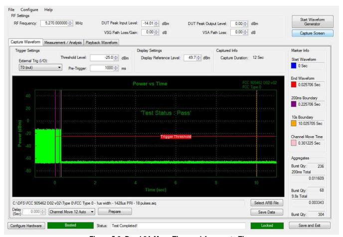
Figure 5-3. Band 2A Move Time and Aggregate Time
