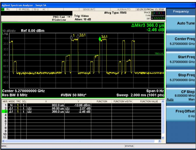
Figure 5-1. Band 2A Pulse Width and Period
