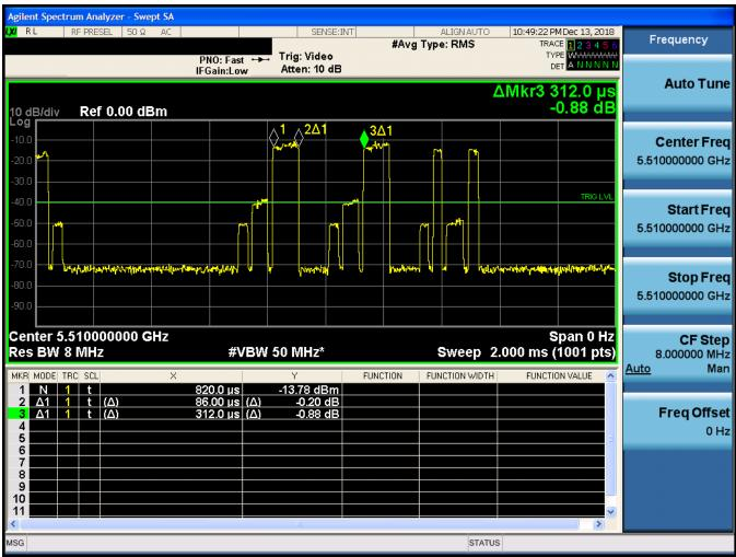
Figure 5-2. Band 2C Pulse Width and Period
